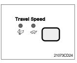
This switch is to control the travel speed which is changed to high speed(Rabbit mark) by pressing the switch and low speed(Turtle mark) by pressing again.
