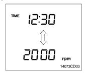
This displays the current time and machine information such as engine rpm, coolant/hydraulic oil temperature, hydraulic oil pressure and also error codes.
