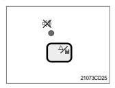
When the starting switch is turned ON first, normally the alarm buzzer sounds for 5 seconds during lamp check operation.
