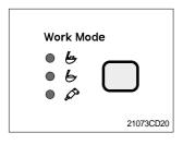
This switch is to select the machine operation mode, which shifts from general operation mode to heavy operation mode and breaker mode in a raw by pressing the switch.
