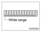
This gauge indicates the amount of fuel in the fuel tank.
