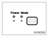
The lamp of selected mode is turned ON by pressing the switch( ), when selecting the mode to use.
