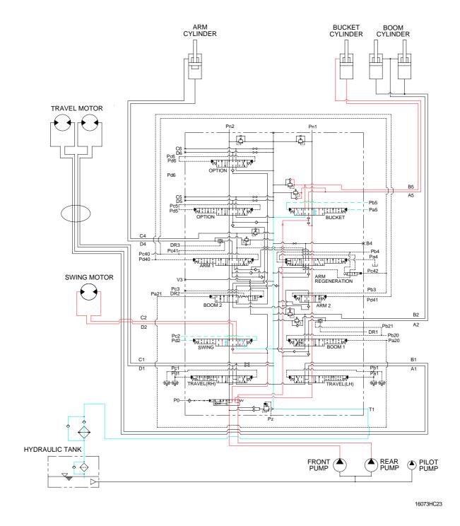
When the swing and bucket functions are operated, simultaneously the swing spool and bucket spool in the main control valve are moved to the functional position by the pilot oil pressure from the remote control valve.
