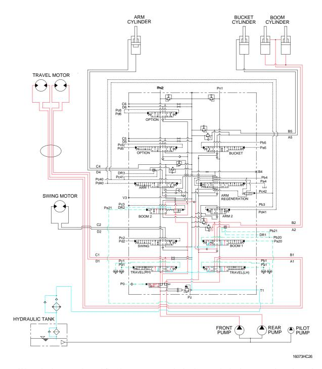
When the boom and travel functions are operated, simultaneously the boom spools and travel spools in the main control valve are moved to the functional position by the pilot oil pressure from the remote control valve and the straight travel spool is pushed to the left by the oil pressure from pilot pump.
