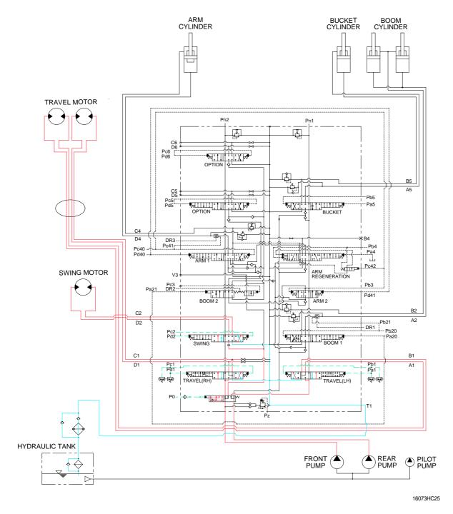
When the swing and travel functions are operated, simultaneously the swing spool and travel spools in the main control valve are moved to the functional position by the pilot oil pressure from the remote control valve and straight travel spool is pushed to the left by the pilot oil pressure from the pilot pump.
