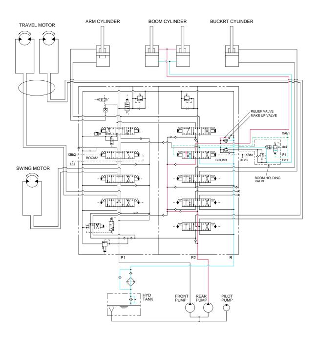
When the right control lever is pushed forward, the boom spools in the main control valve are moved to the lower position by the pilot oil pressure from the remote control valve.
