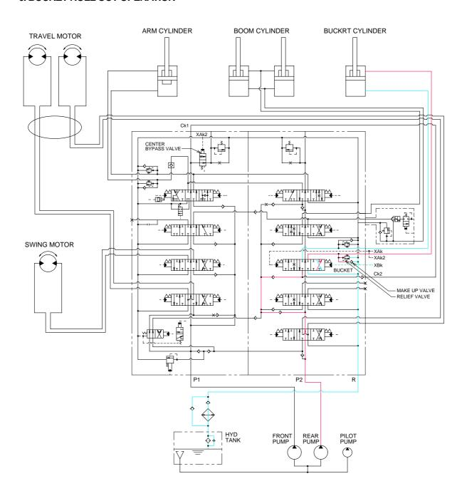
When the right control lever is manually placed in the bucket roll out position. Then the oil flows from pilot pump through the pilot valve to bucket section of the main control valve. Here the spool position is moved to bucket roll out position.
