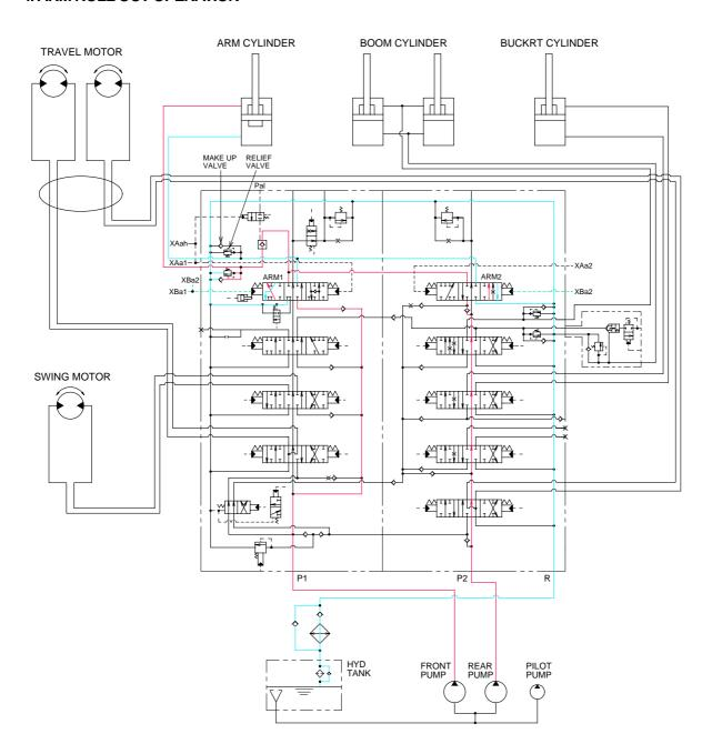
When the left control lever manually is placed in the arm roll out position.
