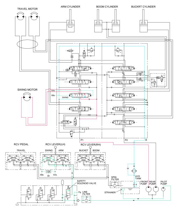
When the left control lever is manually placed in the left(Right) swing position. Then the oil flows from front pump through the swing section of the main control valve to swing motor to left(Right) swing the superstructure. The return oil flows from swing motor through the swing section of the main control valve returned to the tank.
