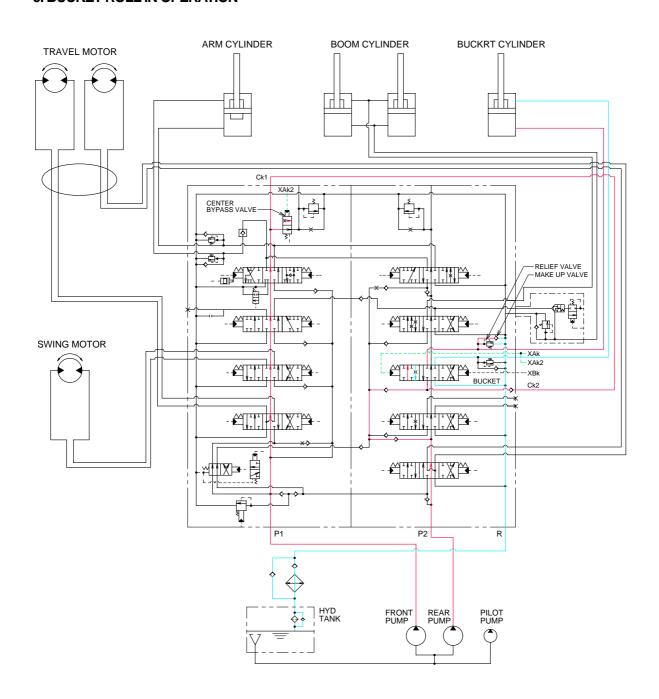
When the right control lever is manually placed in the bucket roll in position. Then the oil flows from pilot through the pilot valve to bucket section of the main control valve. Here the spool position is moved to bucket roll in position.
