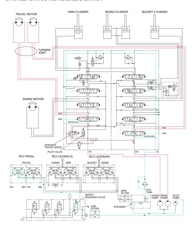
When the right and left travel levers are manually placed to the forward or reverse position, the oil flows from pilot pump through the pilot valve to travel sections of the main control valve.
