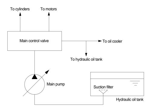
The pumps receive oil from the hydraulic tank through a suction filter. The discharged oil from the pump flows into the control valve and goes out the tank ports.
