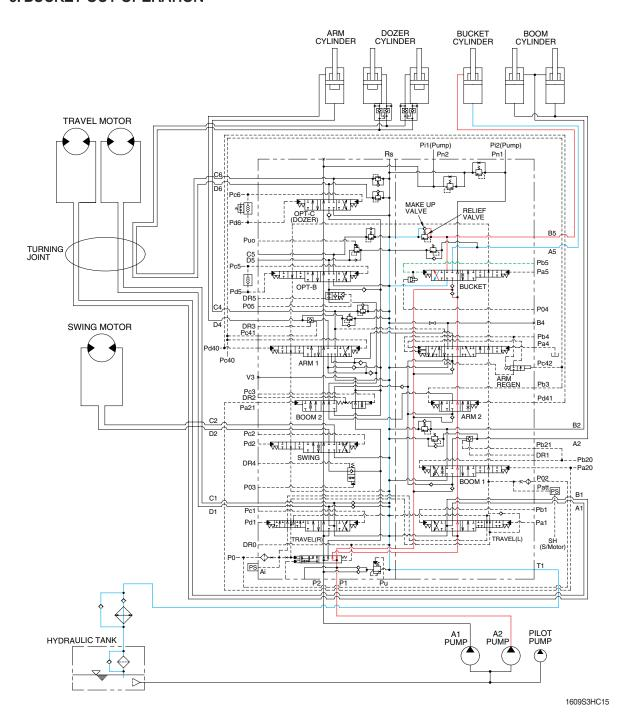
When the right control lever is pushed right, the bucket spool in the main control valve is moved to the bucket out position by the pilot oil pressure from the remote control valve.
