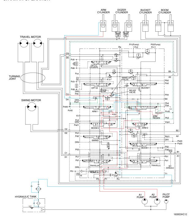
When the left control lever is pulled back, the arm spools in the main control valve are moved to the arm in position by the pilot oil pressure from the remote control valve.
