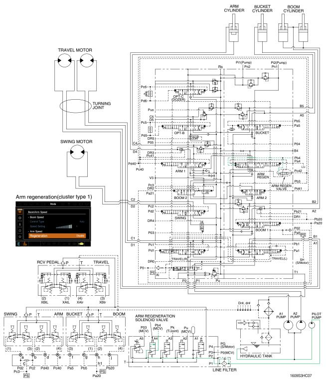
When the arm regeneration is selected to disable on the cluster, the arm regeneration solenoid valve is activated. The pilot oil from pilot pump flows into **Pb4** port in main control valve through solenoid valve and the arm regeneration spool is shifted to left.
