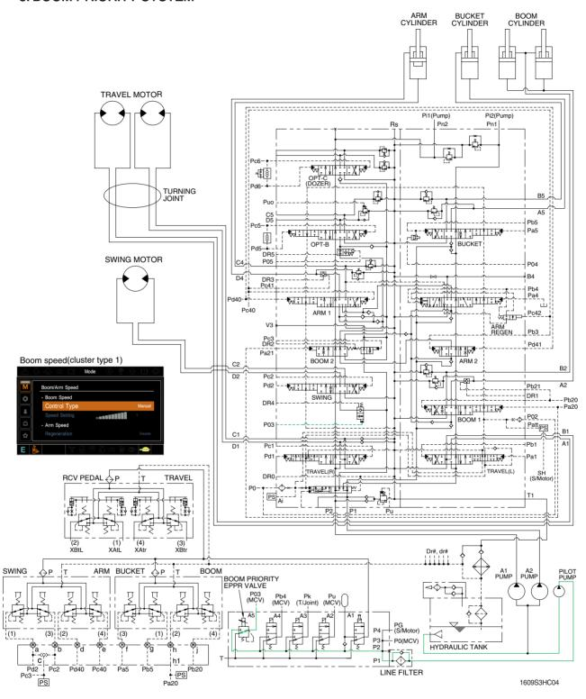
When carrying out the combined operation of swing and boom up, the boom up operating speed is slower than normal operation.
