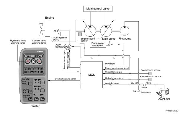
1. If the engine coolant temperature or the hydraulic oil temperature is overheated over 100°C, the warning lamp is ON and the pump input torque or the engine speed is reduced as below logic table.
