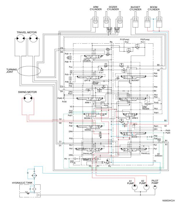
When the swing and boom up functions are operated, simultaneously the swing spool and boom spools in the main control valve are moved to the functional position by the pilot oil pressure from the
