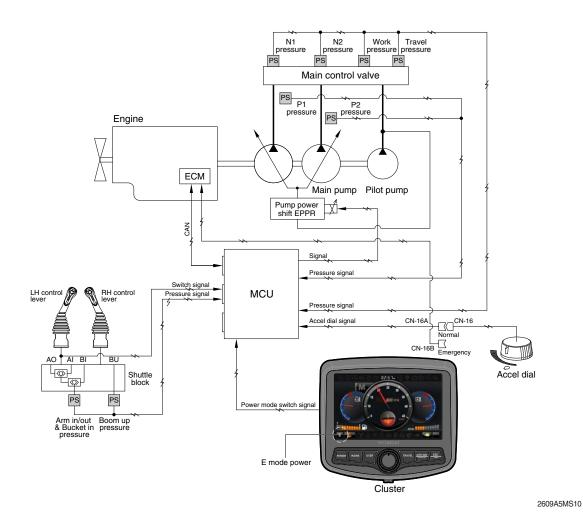
The variable power control system controls the engine and pump mutual power according to RCV lever stroke and pump load.
