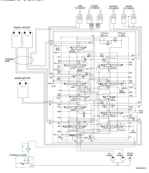
When the dozer control lever is pulled back, the dozer spool in the main control valve is moved to the dozer up position by the pilot oil pressure from the remote control valve.
