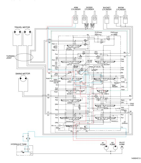
When the left control lever is pushed forward, the arm spools in the main control valve are moved to the arm out position by the pilot oil pressure from the remote control valve.
