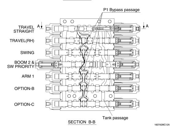
The hydraulic fluid from pump A1 flows into the main control valve through the inlet port "P1", pass the
