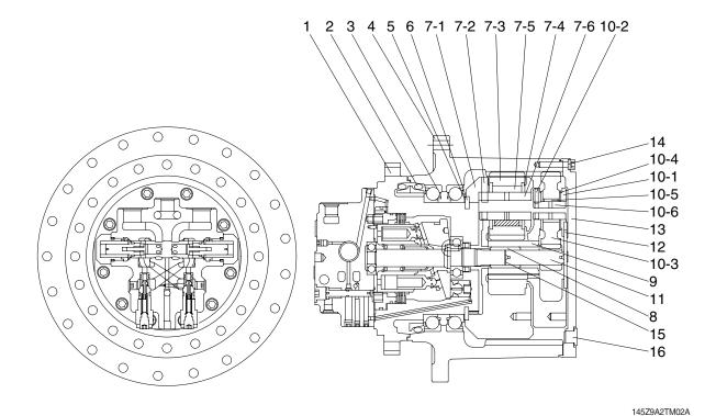
Spindle 7-4 Washer 2 10-5 Bearing 1 1 10-6 Pin 1 2 Floating sesal 7-5 Bearing 2 3 Ball bearing 7-6 Pin 2 11 Sun gear 1 4 8 Coupling Plate 1 Housing 12 5 Shim 9 Sun gear 2 Cover 13 6 Shim 10 Carrier assy 1 14 Bolt 7 Carrier assy 2 10-1 Carrier 1 Snap ring 7-1 Carrier 2 10-2 Spring pin 1 Plug 16 7-2 Spring pin 2 10-3 Planetary gear 1
