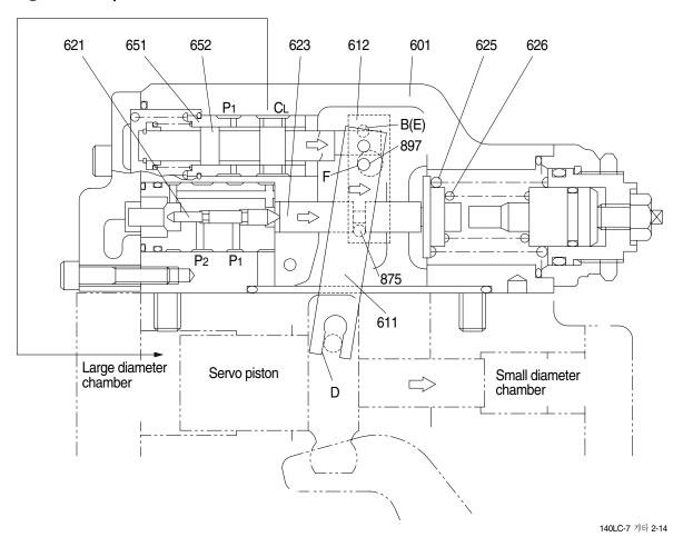
When the self pump delivery pressure P1 or the companion pump delivery pressure P2 rises, it acts on the stepped part of the compensating piston(621). It presses the compensating rod(623) to the right till the force of the outer spring(625) and inner spring(626) balances with the hydraulic force. The movement of the compensating rod is transmitted to lever 1(612) via pin(875). Lever 1 rotates around the pin(875) (E) fixed to the casing(601).
