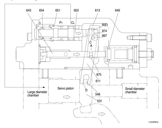
As the pilot pressure Pn rises, the pilot piston(643) moves to the right to a position where the force of the pilot spring(646) balances with the hydraulic force.
