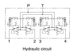
Port size Port Port Ρ Pilot oil inlet port Τ Pilot oil return port Travel (LH, Forward) 1 PF 1/4 2 Travel (LH, Backward) 3 Travel (RH, Forward) 4 Travel (RH, Backward)
