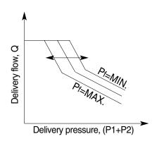
This function permits arbitrary setting of the pump output power, thereby providing the optimum power level according to the operating condition.
