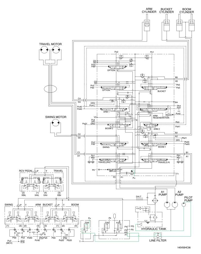
When the power boost switch on the left control lever is pushed ON, the power boost solenoid valve is actuated, the discharged oil from the pilot pump flows into Pu port of the main relief valve of main control valve; then the setting pressure of the main relief valve is raised from 330kgf/cm<sup>2</sup> to 360kgf/cm<sup>2</sup> for increasing the digging power. And even when pressed continuously, it is canceled after 8 seconds.
