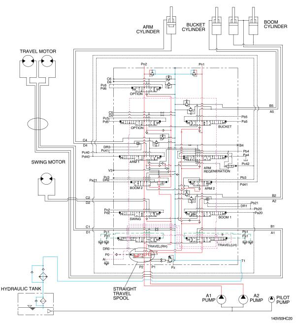
The oil from the A1 and A2 pump flows through the neutral oil passage, bypass oil passage and confluence oil passage in the main control valve. Then the oil goes to each actuator and operates them. Check valves and orifices are located on these oil passage in the main control valve. These control the oil from the main pumps so as to correspond to the operation of each actuator and smooth the combined operation.
