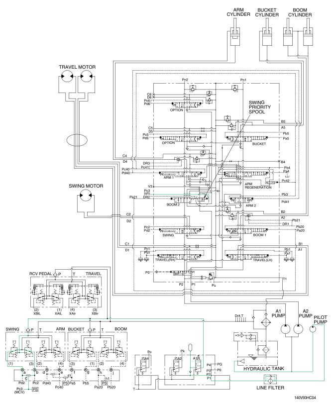
When carrying out the combined operation of swing and boom or arm of the left control valve, the swing speed can be lowered than operating speed of boom or arm. To prevent it, swing priority spool is used. Pc3 pressure from shuttle valve(sh) shifts the swing priority spool to the left and decreases the oil flow rate to the boom or arm section by orifice.
