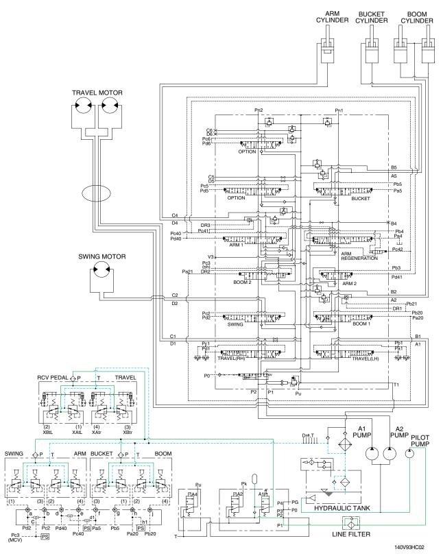
The pilot pump receive oil from the hydraulic tank. The discharged oil from the pilot pump flows to the safety solenoid value through the line filter. The oil is filtered by the line filter. The pilot relief value is provided in the pilot pump for limiting the pilot circuit pressure.
