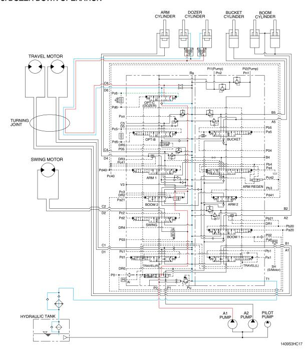
When the dozer control lever is pushed forward, the dozer spool in the main control valve is moved to the dozer down position by the pilot oil pressure from the remote control valve.
