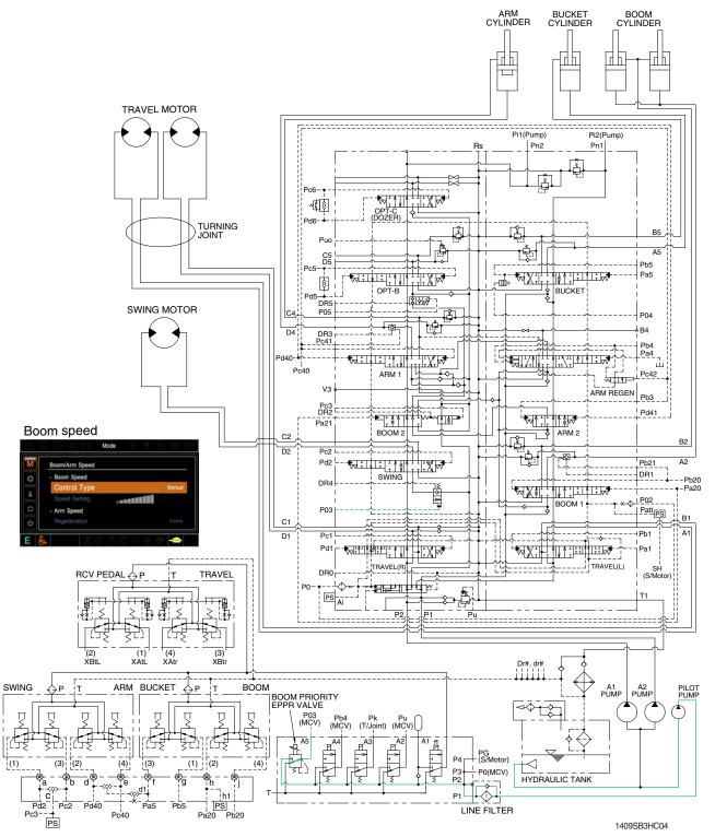
When carrying out the combined operation of swing and boom up, the boom up operating speed is slower than normal operation.
