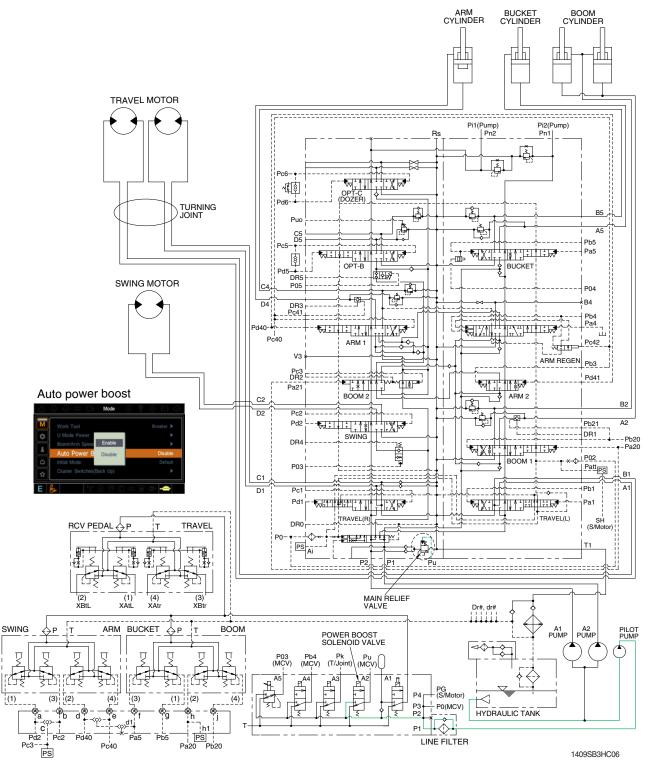
When the power switch on the left control lever is pushed ON, the power solenoid valve is actuated, the discharged oil from the pilot pump flows into **Pu** port of the main relief valve of main control valve; then the setting pressure of the main relief valve is raised from 350 kgf/cm<sup>2</sup> to 380 kgf/cm<sup>2</sup> for increasing the digging power.
