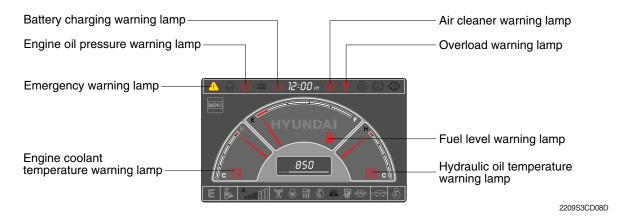
Each warning lamp on the top of the LCD pops up on the center of LCD and the buzzer sounds when the each warning is happened. The pop-up warning lamp moves to the original position and blinks when the select switch is pushed. And the buzzer stops.
