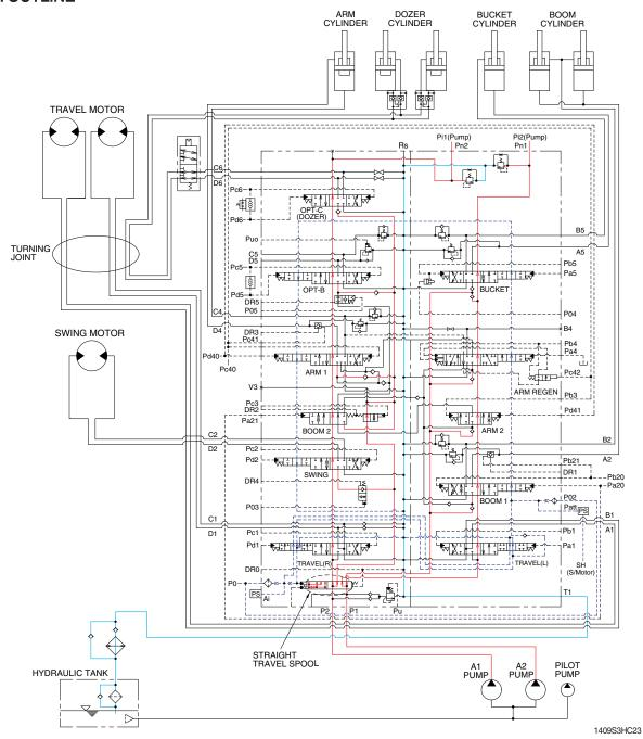
The oil from the A1 and A2 pump flows through the neutral oil passage, bypass oil passage and confluence oil passage in the main control valve. Then the oil goes to each actuator and operates them. Check valves and orifices are located on these oil passage in the main control valve. These control the oil from the main pumps so as to correspond to the operation of each actuator and smooth the combined operation.
