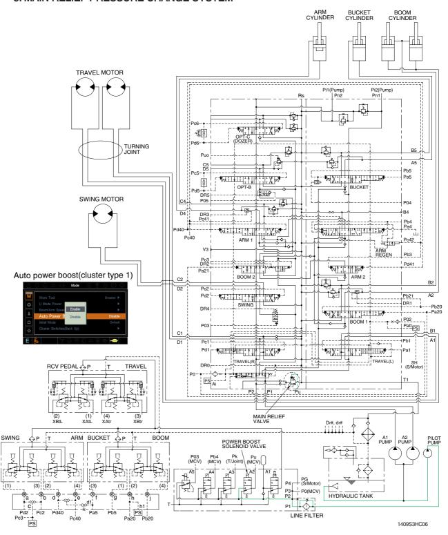
When the power switch on the left control lever is pushed ON, the power solenoid valve is actuated, the discharged oil from the pilot pump flows into Pu port of the main relief valve of main control valve; then the setting pressure of the main relief valve is raised from 350 kgf/cm² to 380 kgf/cm² for increasing the digging power.
