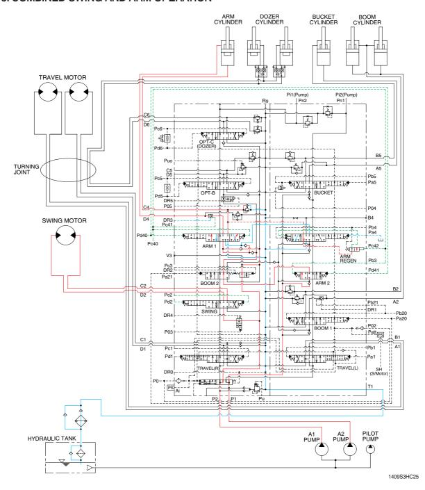
When the swing and arm functions are operated, simultaneously the swing spool and arm spools in the main control valve are moved to the functional position by the pilot oil pressure from the remote control valve.
