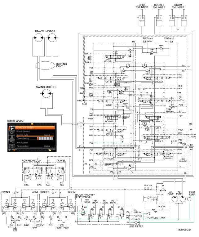
When carrying out the combined operation of swing and boom up, the boom up operating speed is lowered than normal operation.
