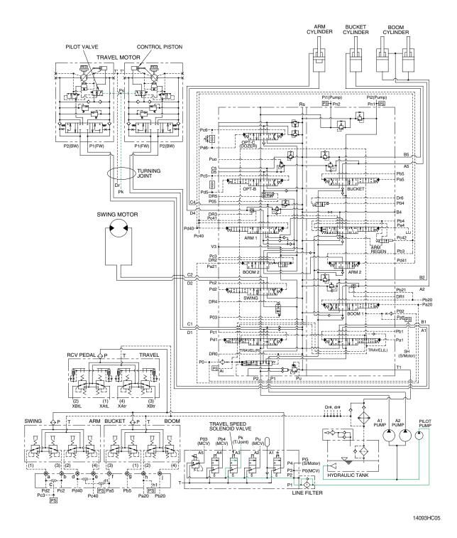
When the travel speed switch is pushed, the travel speed solenoid valve is actuated and the discharged oil from the pilot pump flows to the **Ps** port of pilot valve in the travel motors. As a result, the control piston is pushed by the main oil flow, thus the displacement is minimized. When the travel speed switch is pushed once more, the travel speed solenoid valve is return to
