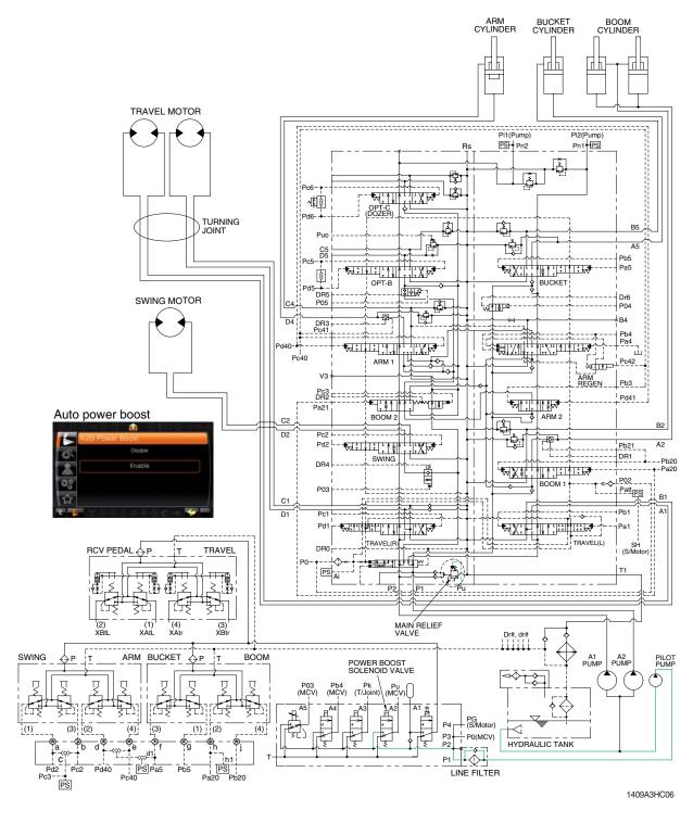
When the power switch on the left control lever is pushed ON, the power solenoid valve is actuated, the discharged oil from the pilot pump flows into **Pu** port of the main relief valve of main control valve; then the setting pressure of the main relief valve is raised from 350 kgf/cm² to 380 kgf/cm² for increasing the digging power.
