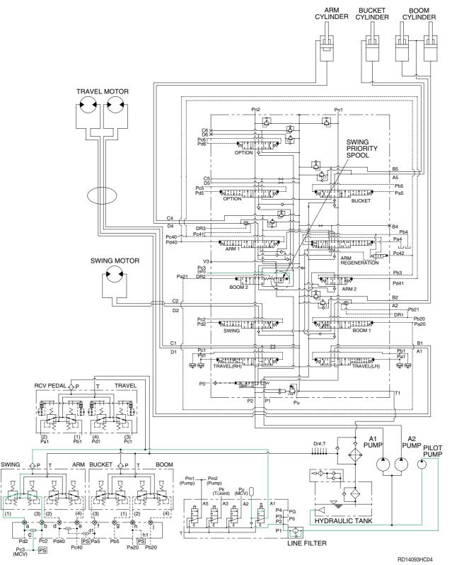
When carrying out the combined operation of swing and boom or arm of the left control valve, the swing speed can be lowered than operating speed of boom or arm. To prevent it, swing priority spool is used. Pc3 pressure from shuttle valve(sh) shifts the swing priority spool to the left and decreases the oil flow rate to the boom or arm section by orifice. This is called the swing priority system.
