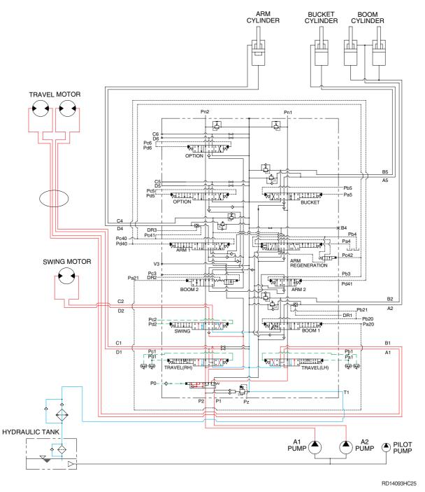
When the swing and travel functions are operated, simultaneously the swing spool and travel spools in the main control valve are moved to the functional position by the pilot oil pressure from the remote control valve and straight travel spool is pushed to the left by the pilot oil pressure from the
