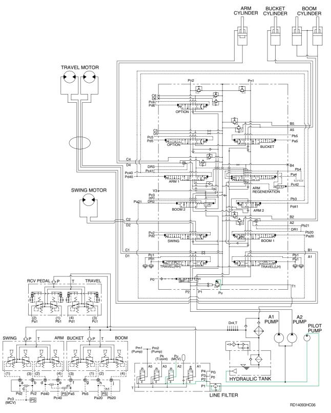
When the power boost switch on the left control lever is pushed ON, the power boost solenoid valve is actuated, the discharged oil from the pilot pump flows into Pu port of the main relief valve of main control valve; then the setting pressure of the main relief valve is raised from 330kgf/cm2 to 360kgf/ cm2 for increasing the digging power. And even when pressed continuously, it is canceled after 8 seconds.
