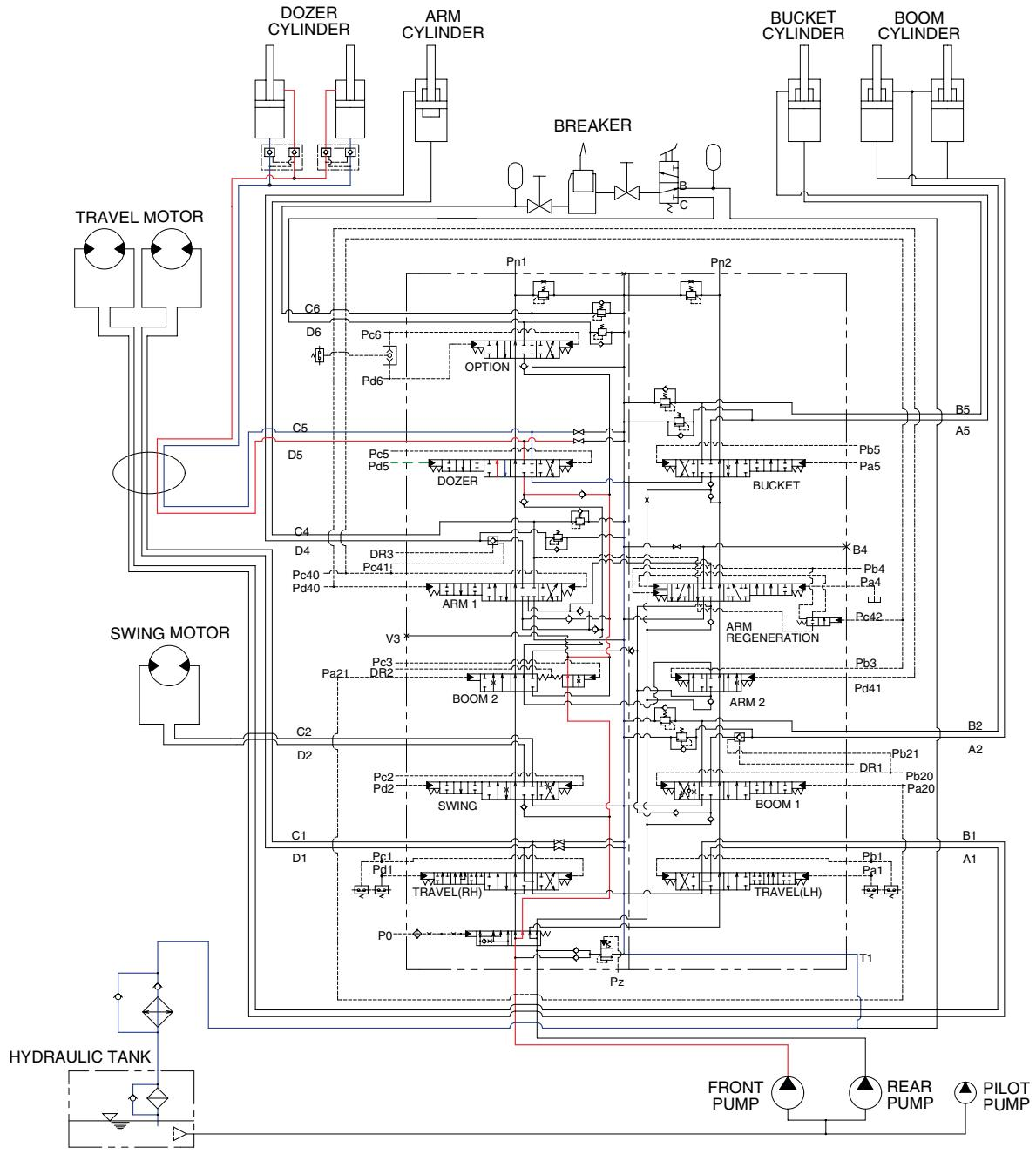
When the dozer control lever is pulled back, the dozer spool in the main control valve is moved to the dozer up position by the pilot oil pressure from the remote control valve.
