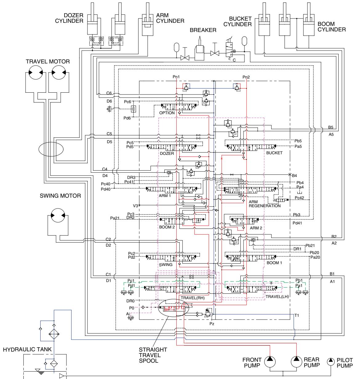
The oil from the front and rear pump flows through the neutral oil passage, bypass oil passage and confluence oil passage in the main control valve. Then the oil goes to each actuator and operates them. Check valves and orifices are located on these oil passage in the main control valve. These control the oil from the main pumps so as to correspond to the operation of each actuator and smooth the combined operation.
