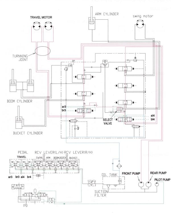
When the right and left travel levers are manually placed to the forward or reverse position. Then the oil flows from front pump through the travel(R) section of the control valve and turning joint to the right travel motor and oil flows from rear pump through the travel(L) section of the control valve and turning joint to the left travel motor and move the machine forward and reverse.
