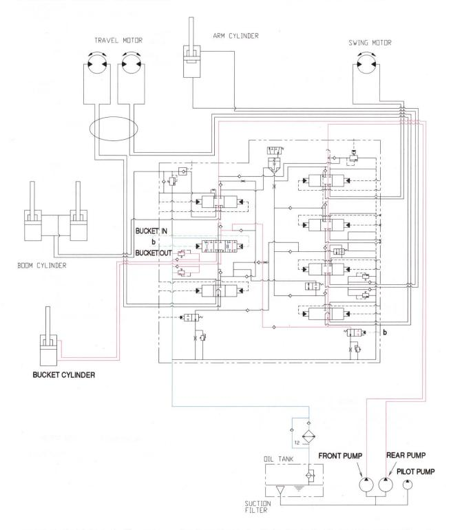
When the right control lever manually placed in the bucket roll in(roll out) position. Then the oil from pilot pump through the pilot valve to bucket section of the control valve. Here the spool position is moved to bucket roll in(roll out) position.
