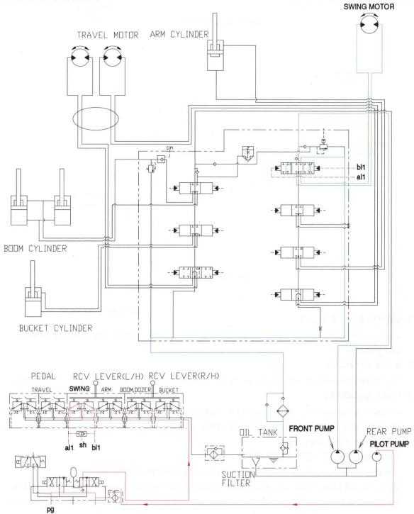
When the left control lever is manually placed in the left(right) swing position. Then the oil flows from front pump through the swing section of the control valve to swing motor to left(right) swing the superstructure. The return oil flow from swing motor through the swing section of the control valve returned to the tank.
