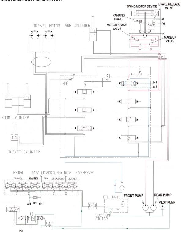
When the left control lever manually is placed in the swing positon. Then the oil flows from pilot pump through the pilot valve to the swing section of the control valve. Here, the spool position is moved to right or left swing position.
