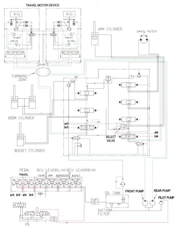
When the travel levers are manually placed to the forward or reverse position.
