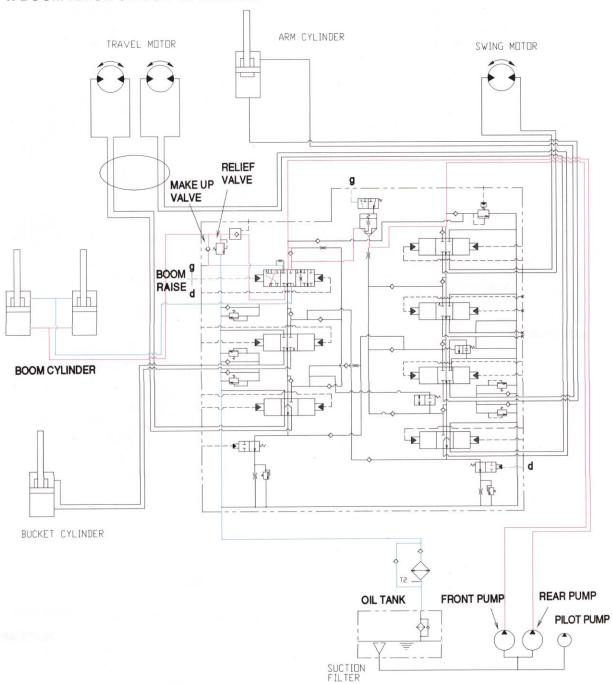
When the right control lever is pulled to boom raise position. Then the oil from pilot pump through the remote control valve to boom sections of the control valve.
