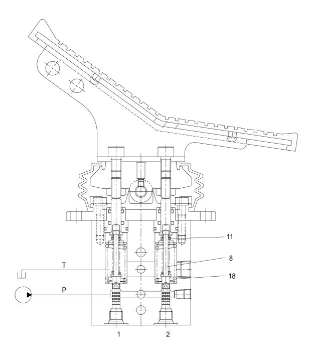
The force of the spring (11) that determines the output pressure of the pilot valve is not applied to the spool (8). Therefore, the spool is pushed up by the spring (18) to the position of port 2 in the operation explanation drawing. Then, since the output port is connected to tank port T only, the output port pressure becomes equal to tank pressure.
