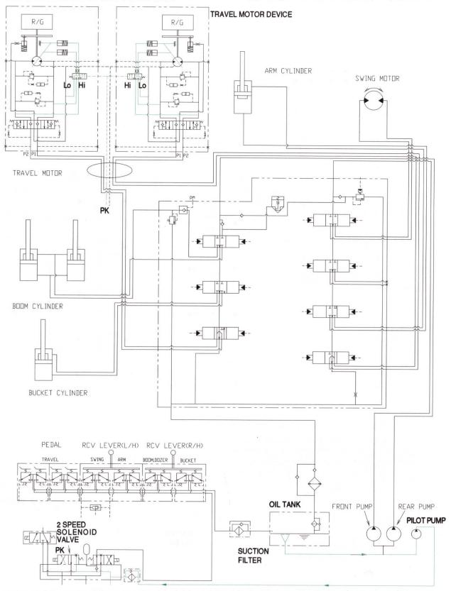
When the travel speed solenoid valve was placed in the HI position, the pressure oil from pilot pump flows to PK port of 2 speed change over valve, and the control piston is pushed up, thus minimizing the displacement.
