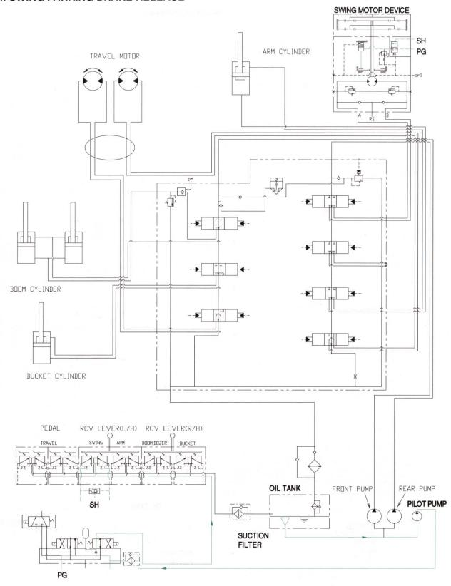
When the swing control lever is tilted, the pilot oil go to SH port of shuttle valve, this pressure move spool so, discharged oil from pilot pump go to PG port.
