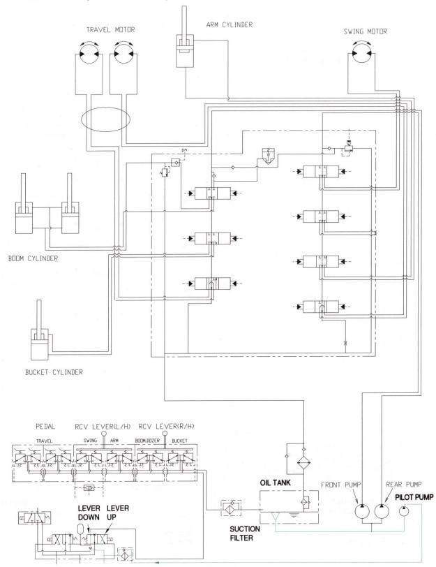
When the lever of the safety solenoid valve moved downward, oil flow remote control valve through solenoid valve.
