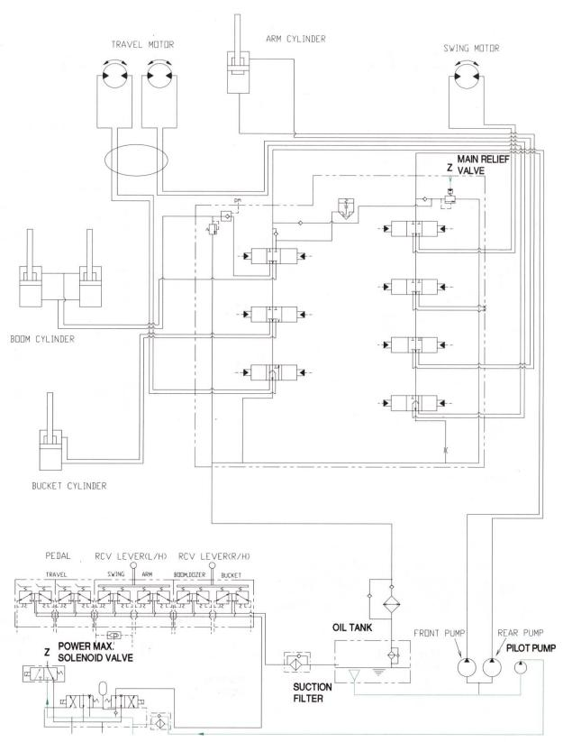
When the power max switch keeps pressed, the main relief valve pressure changes from  $320\,kg/m^2$  to  $350\,kg/m^2$  for maximum 8 seconds.
