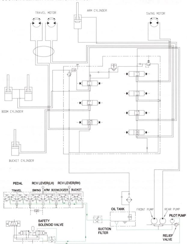
The pilot pump receive oil from the hydraulic tank through a suction filter. The discharged oil from the pilot pump flows to the safety solenoid valve through the pilot filter. The oil is filtered by the pilot filter. The pilot relief valve is provided in the pilot pump for limiting the pilot circuit pressure. The oil filtered by pilot filter flows remote control valve through safety solenoid valve.
