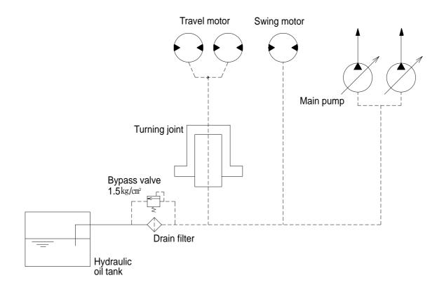
Besides internal leaks from the motors and main pump, the oil for lubrication circulates. These oil have to be fed to the hydraulic tank passing through drain filter.
