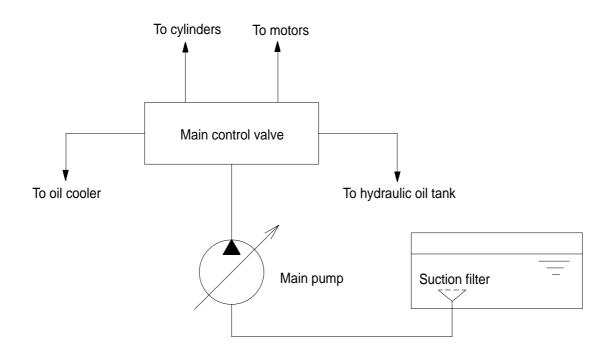
The pump receive oil from the hydraulic tank through a suction filter. The discharged oil from the pump flows into the control valve and goes out the tank ports.
