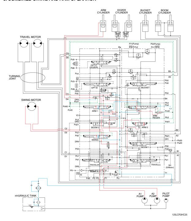
When the swing and arm functions are operated, simultaneously the swing spool and arm spools in the main control valve are moved to the functional position by the pilot oil pressure from the remote
