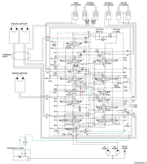
When the dozer control lever is pushed forward, the dozer spool in the main control valve is moved to the dozer down position by the pilot oil pressure from the remote control valve.
