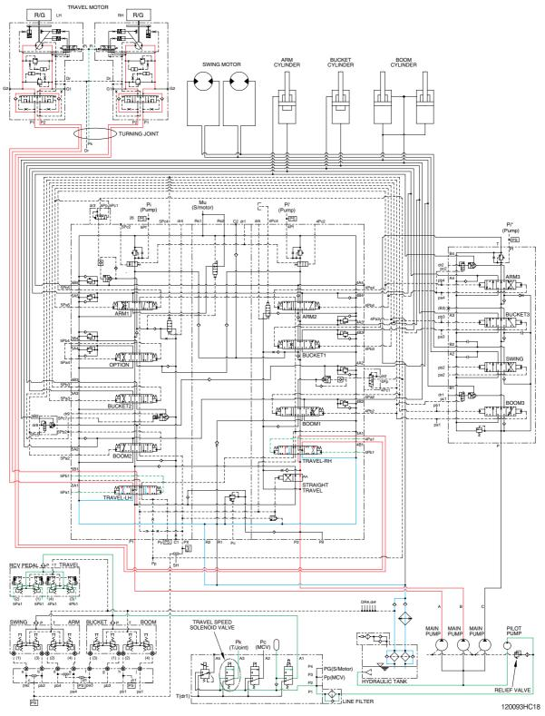
When the travel levers are pushed forward or reverse position, the travel spools in the main control valve are moved to the forward or reverse travel position by the pilot oil pressure from the remote control valve.
