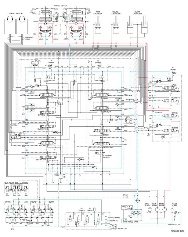
When the LH control lever is pushed left or right, the swing spool in the main control valve 2 is moved to the left or right swing position by the pilot oil pressure from the remote control valve.
