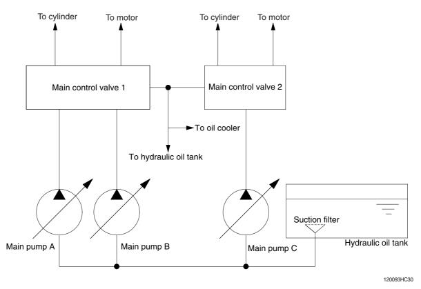
The pumps receive oil from the hydraulic tank through a suction filter. The discharged oil from the pump flows into the control valve and goes out the tank ports.
