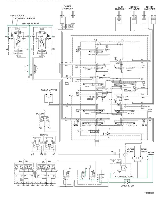
When the travel speed switch is pushed, the travel speed solenoid valve is actuated and the discharged oil from the pilot pump flows to the Pk port of pilot valve in the travel motors.
