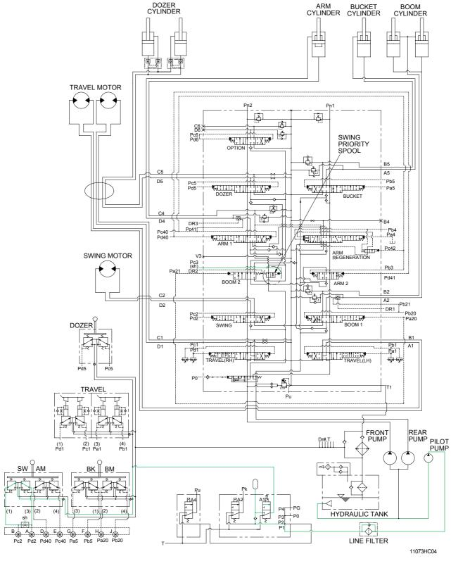
When carrying out the combined operation of swing and boom or arm of the left control valve, the swing speed can be lowered than operating speed of boom or arm. To prevent it, swing priority spool is used. Pc3 pressure from shuttle valve(sh) shifts the swing priority spool to the left and decreases the oil flow rate to the boom or arm section by orifice.
