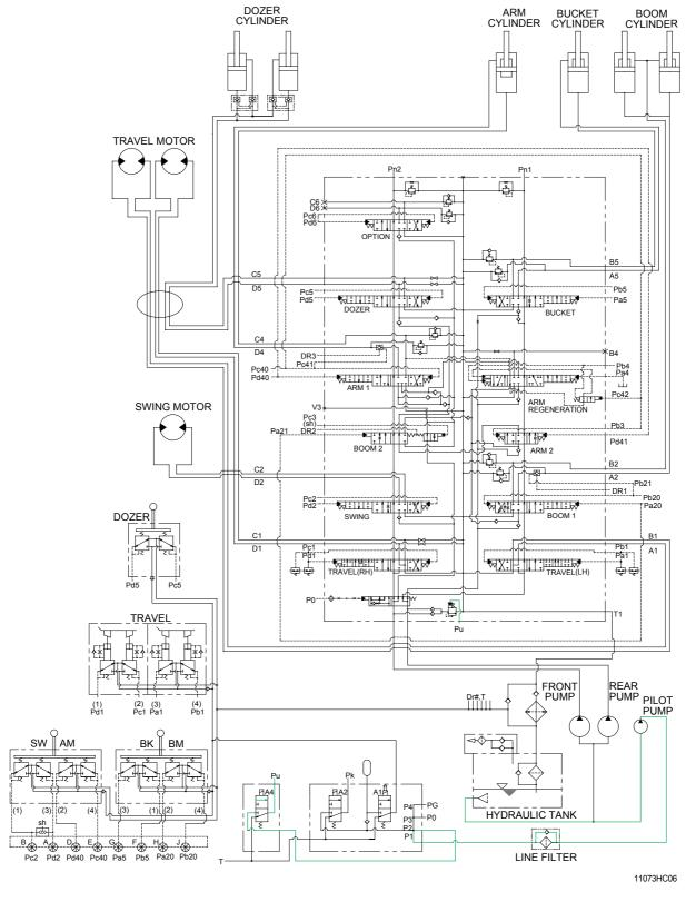
When the power boost switch on the left control lever is pushed ON, the power boost solenoid valve is actuated, the discharged oil from the pilot pump flows into Pu port of the main relief valve of main control valve; then the setting pressure of the main relief valve is raised from 330kgf/cm² to 360kgf/cm² for increasing the digging power. And even when pressed continuously, it is canceled after 8 seconds.
