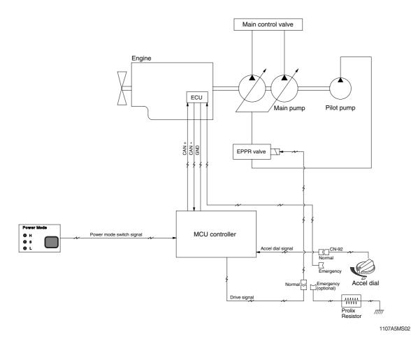
Mode selection system(Micro computer based electro-hydraulic pump and engine mutual control system) optimizes the engine and pump performance.
