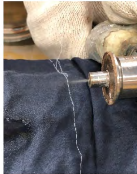
Illustration 76 g06550349 Example of a good injector spray pattern
