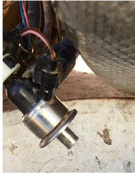
Illustration 124 Typical example of droplets forming on the DEF injector nozzle
