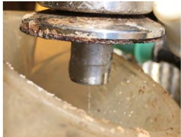
Illustration 77 g06550358 Example of a poor DEF injector spray pattern
