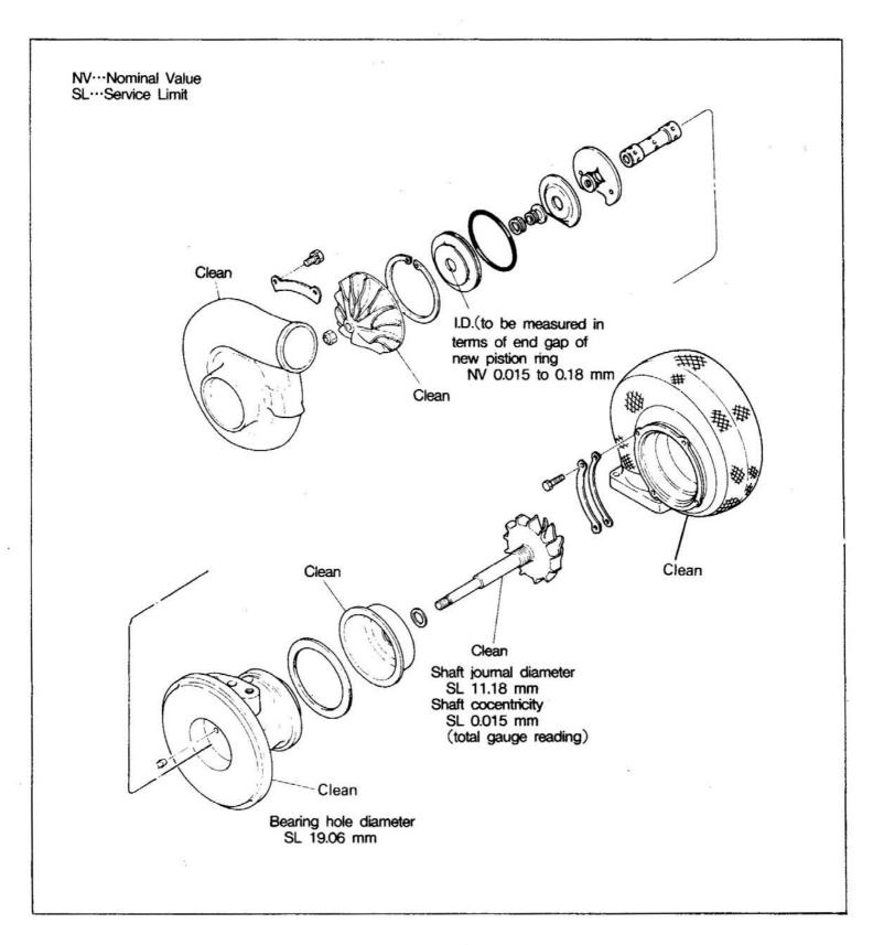
NOTE: The parts may be cleaned by use of a blast equipment or any other effective methods, but a non-corrosive neutral detergent should be used.
