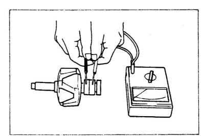
If the slip ring has rough surface or unevenly worn surface, correct with sandpaper or lathe.
