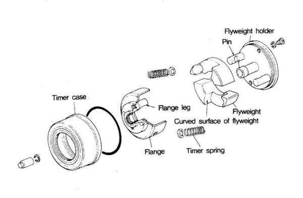
The two flyweights have a hole at one end. The pins of the flyweight holder fit in the holes. The flange legs touch the curved surfaces of the flyweights. Timer springs are mounted to the flyweight pins and flange legs.
