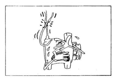
(6) When the battery is to be quick-charged with a quick charger, be sure to disconnect the battery terminal connections beforehand. Otherwise, the diode and the regulator would be damaged.
