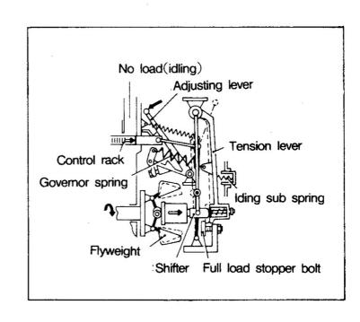
that fuel is reduced, thereby preventing the engine from exceeding the specified speed.
