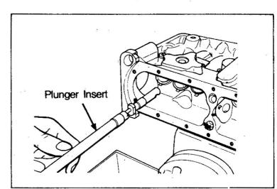
(m) Remove the upper spring seat 15 and control sleeve 16. The control sleeve can be easily removed by use of special tool(Plunger Clamp Device).
