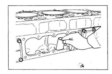
(6) Seat the cylinder head 10 on the crankcase, while lining it up with the locating pin.
