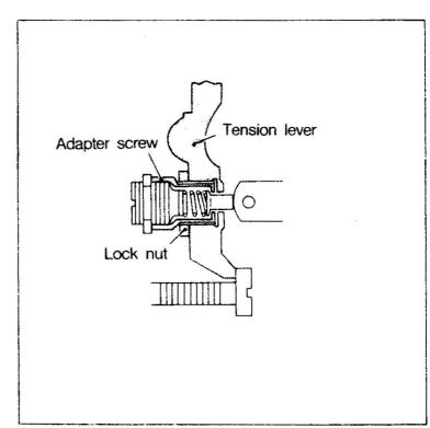
Tightening the adapter screw will increase the ungleich stroke.
