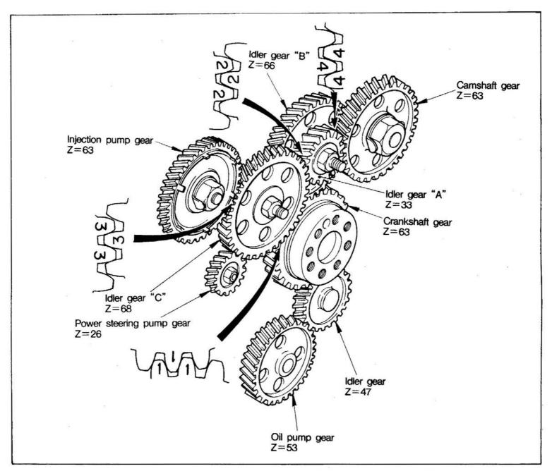
Each gear is a carbon steel helical gear. The tooth surfaces are machined by shaving to form close-tolerance tooth profile, and are given surface treatment to offer improved durability. A timing mark is stamped on each timing gear. Correct meshing can be achieved by aligning the timing marks at reassembly.
