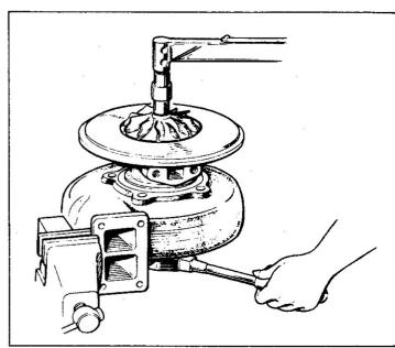
(9) Set a dial indicator on the turbine wheel shaft end. Move the compressor wheel up and down to measure the end play. If the play is out of specification, desassemble and check to locate the cause.
