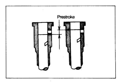
If the prestroke is out of specification, adjust by changing the shim thickness between the flange sleeve and pump housing.
