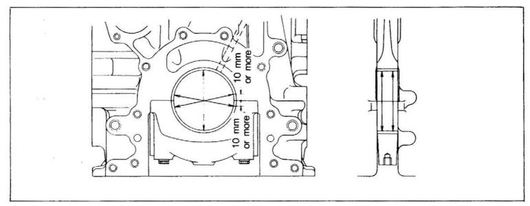
(2) Measure the free time tension of the main bearing. If the tension is below the service limit, replace the upper and lower bearings as a set.
