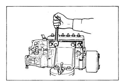
(d) Remove the cover 1 and remove the lock nut 2 with special tools (Socket Wrench and Handle).
