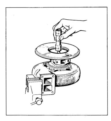
(4) Apply engine oil to both sides of the thrust bearing 10 and thrust ring 9 before assembling them on the turbine wheel shaft. Then install the oil deflector 8.
