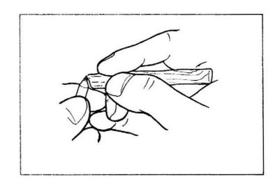
(b) Pass a cleaning needle through the injection orifice of the nozzle, while turning the needle, to remove carbon.
