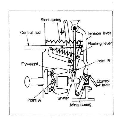
At the same time, the fulcrum B will also slightly move toward the pump housing to push the control rod back in the direction for decreasing the fuel injection rate.
