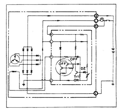
When the generated voltage falls too far below the Zener voltage, "Dz" does not conduct so that "Tr<sub>1</sub>" is forced to the OFF state.
