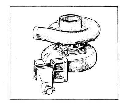
(2) Remove the turbine housing 1.
