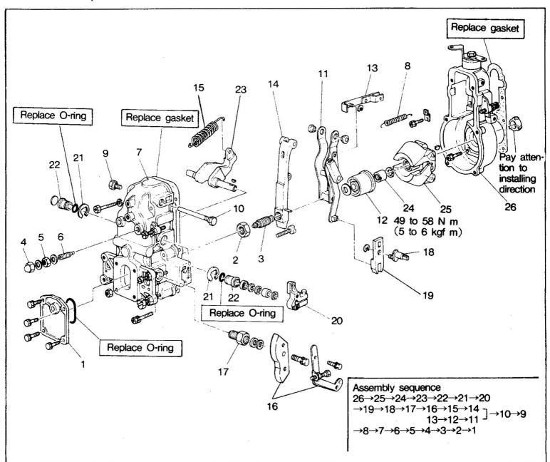
(a) Install the governor housing 26. After installation, remove the special tool(Tappet Holder or Tappet Pin).
