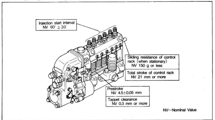
NOTE: Supply oil to the injection pump cam chamber.
