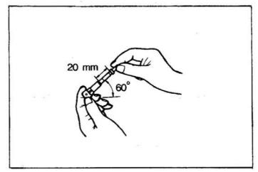
Measure the width between the driving faces of the plunger and the width of the groove in the control sleeve. If the calculated clearance between driving face and groove is in excess of the service limit, replace the control sleeve.
