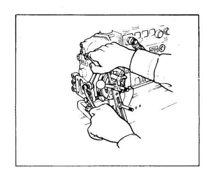
Adjust the idling spring so that when the pump speed is Nc, the control rod will be positioned at R<sub>4</sub>.
