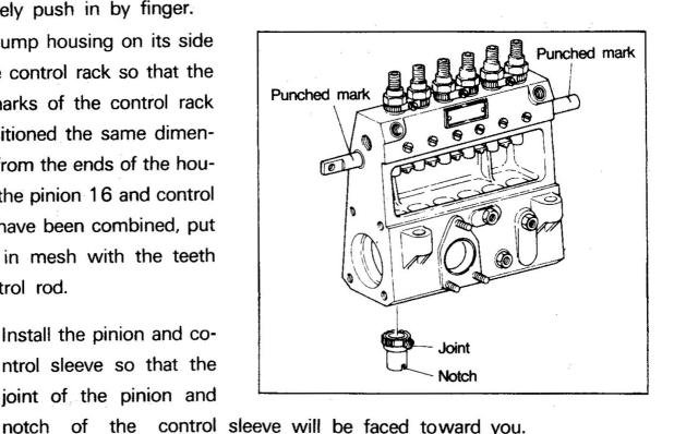
2. After each pinion has been installed, move the control rack to conthat it can be moved the same amount to right and left. firm
