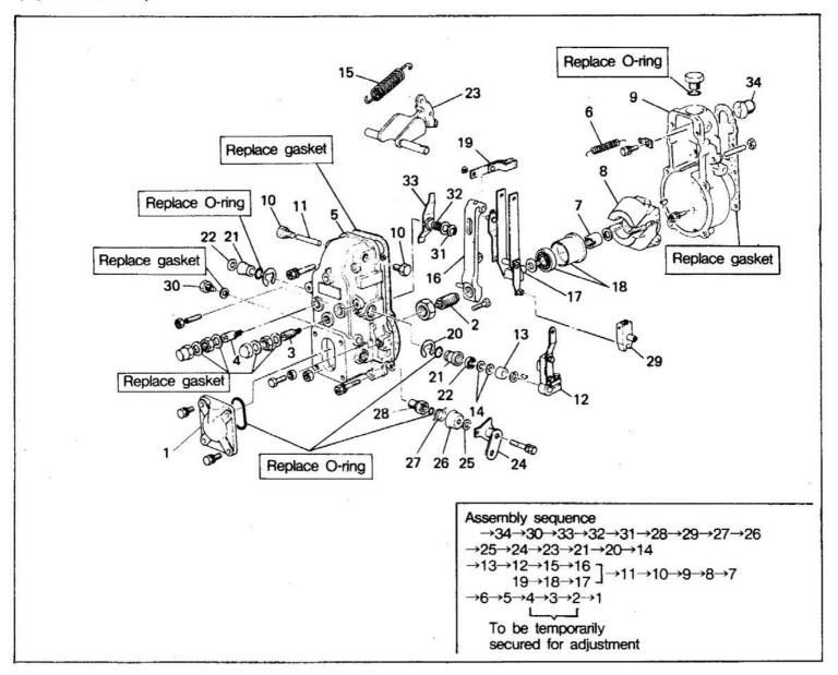
Reassemble the governor by reversing the above-mentioned disassembly procedures.
