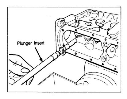
(e) Mount special tool(Tappet Mounting Device) to the pump housing.
