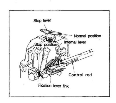
Since the amount the control rod is moved by operation of the stop lever exceeds the operating range of the floating lever mechanism, damage to the link and allied parts is prevented by the cancel mechanism shown.
