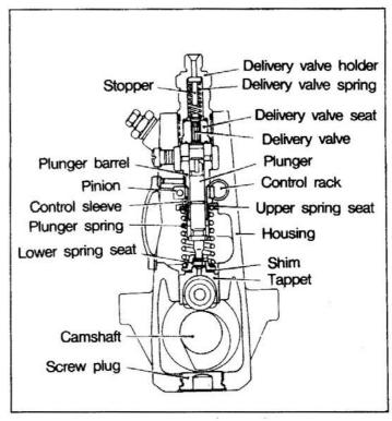
to up-and-down motion which is transmitted to the plunger.
