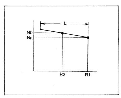
NOTE: If the speed variation rate is poor, the engine will exceed the specified maximum speed at no load and will enter a hazardous condition.
