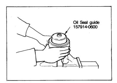
(h) After the oil seal guide has been removed, turn down the timer case onto the holder with special tool (Band Spanner), and punch it.
