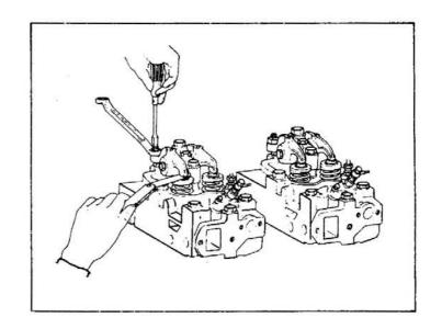
After the clearnce has been adjusted, tighten the lock nut to secure the adjusting screw.
