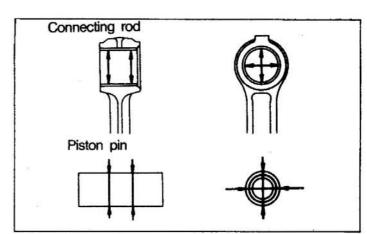
(2) Replacement of Connecting Rod Bushing
