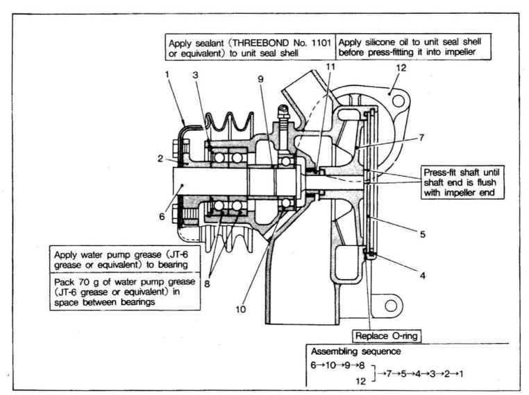
NOTE: After reassembly, turn the water pump pulley by hand to confirm that the impeller does not touch the case and cover.
