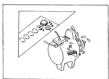
(3) Do not use a high voltage tester such as megger to test the alternator as it could cause damage to the diode and the regulator.
