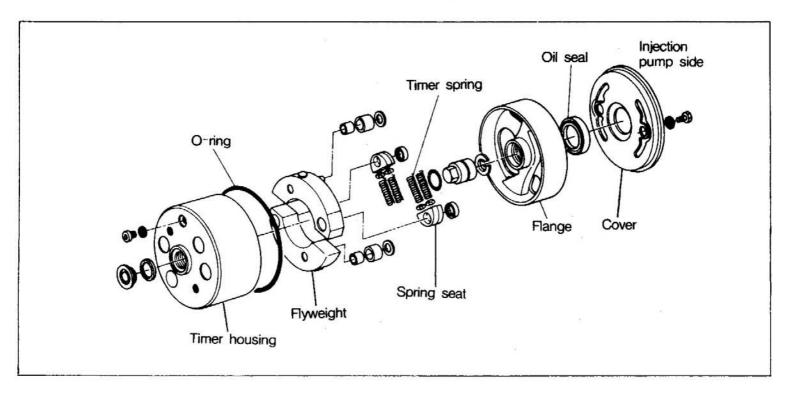
Two flyweights are fitted on the pins of the timer housing and are held in the timer housing. On the other hand, the injection pump connection side flange has a curved surface, and the roller fitted on the pin installed in the flyweight touches the curved surface. Timer springs are held between the spring seats fitted on the timer housing pins which extend through the flange and flyweight. These parts are housed in the timer housing and are totally enclosed with a cover, O-ring and oil seal.
