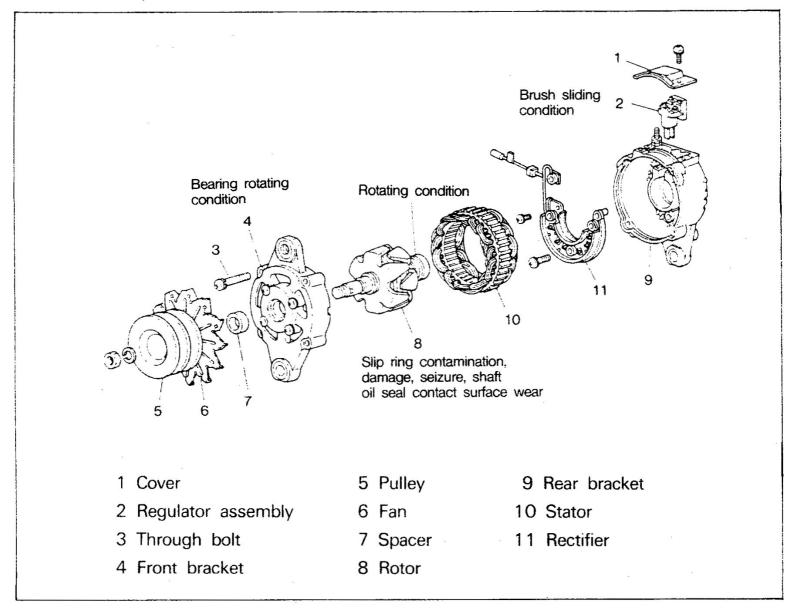
NOTE: 1. If disassembly is continued without removing the regulator assembly, the brush will be damaged when removing the rotor.
