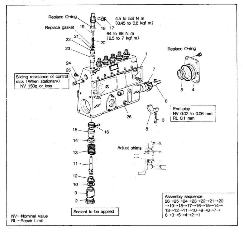
(a) Mount the pump housing 26 in special tool(Universal Vice). After the control rack 25 has been inserted, thread the screw 24 into the back of the pump housing.
