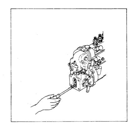
Clockwise rotation of the full load stopper, as viewed from the rear of the governor, will move, the rack in the direction fuel is increased.
