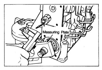
the dimension from the end of the pump housing to the end of the Measuring Plate will be  $13.85\pm0.5$  mm.
