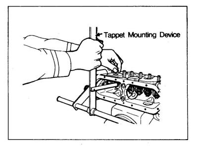
(k) Remove the special tool (Tappet Mounting Device), install a wire in the hole of the lower spring seat 12, pull it together with the plunger until the lower spring seat can be removed, and remove only the lower spring seat.
