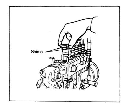
NOTE: To install the plunger block, apply grease to each O-ring. After inserting the O-ring in the lower part of the plunger barrel into the pump housing in advance, apply grease to the skirt portion of the plunger barrel and then install the plunger barrel.
