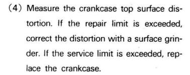
NOTE: When the crankcase is ground, make sure that the piston projection does not exceed the nominal dimension.
