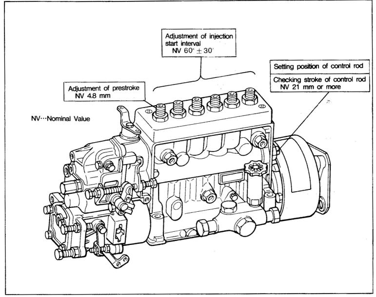
NOTE: 1. Supply oil to the injection pump cam chamber.
