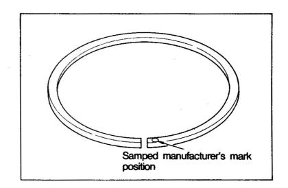
Direct the open ends of the piston rings as shown.
