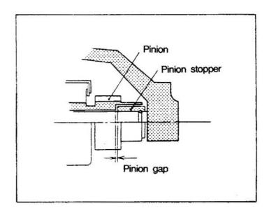
2. The pinion is pushed by a spring in the direction that it moves out. Even if it is pushed back by hand, the pinion will return when released.
