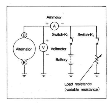
With the load resistance set at maximum(almost no load current flowing), close switches K<sub>1</sub> and K<sub>2</sub>. While increasing the alternator speed gradually, decrease the load resistance and measure the specified terminal voltage and the current value at specified speed.
