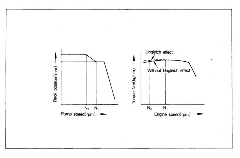
When the engine speed is low and the centrifugal force of flyweight smaller than the pressure of the Ungleich spring, the control block is moved as much as the Ungleich stroke to the left, so the control rack moves in the direction that fuel is increased to increase the torque of the engine at low speeds.
