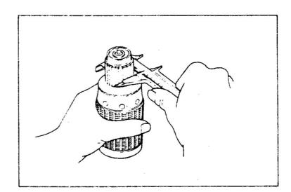
c) Measure the depth of groove between segments. If the depth is less than the repair limit, correct.
