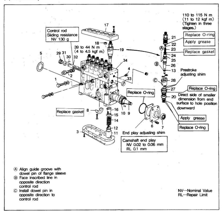
(a) Mount the pump housing 34 in special tool(Universal Vice).
