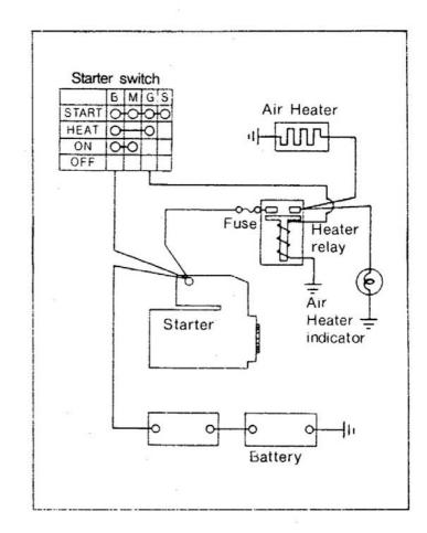
The heater relay is provided with a fuse of the air heater circuit. Check the fuse and replace if burned out, after determining the cause of the burn-out.
