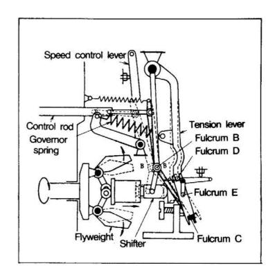
Movement of the point B and movement of the point C will combine to pull the control rod back in the direction of less fuel injection rate, thereby preventing the engine speed from increasing.
