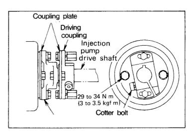
Then tighten the cotter bolt to the specified torque.
