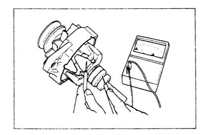
Measure the resistance between the slip rings. Replace the rotor if the resistance is not as specified.
