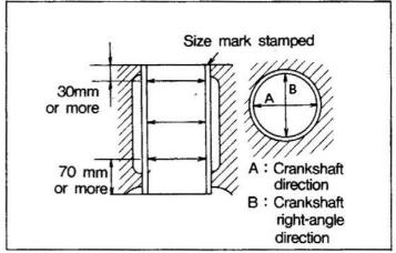
NOTE: When a cylinder liner needs replacing, make sure that the liner with the same size mark as that of the piston is selected.
