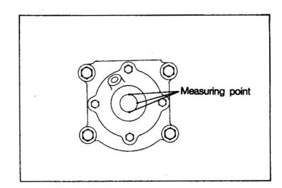
If the eccentricity between the mandrel and injection pump drive shaft is in excess of the nominal dimension, adjust by adding or removing injection pump bracket shims.
