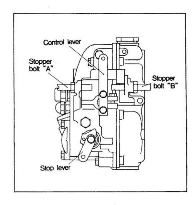
NOTE: After idling adjustment, quickly move the control lever from the full load position to the idling position to verify that the engine does not stall and no hunting occurs. If abnormal condition occurs, make adjustment as far as the specified idling limits allow. If adjustment is impossible, disassemble and inspect the injection pump.
