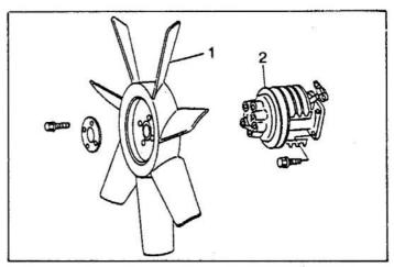
NOTE: Remove or install the fan drive by operating the tension pulley.
