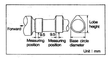
(2) Measure the camshaft journal O.D. and crankcase I.D. If the repair limits are exceeded, the bushing in the crankcase should be replaced.
