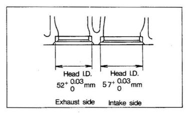
(d) Using Caulking Tool(special tool), install the valve seat insert and caulk the periphery of the valve seat.
