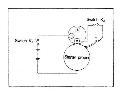
pinion comes out rotating, open the switch K<sub>2</sub> to stop rotation of the pinion.
