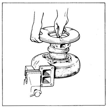
(3) Apply engine oil to the I.D. and O.D. of the bearing 15 before installing the bearing in the bearing housing.
