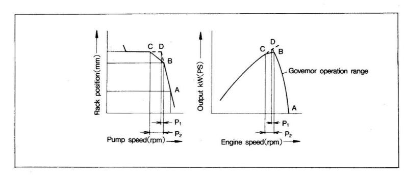
In an abrupt increase of load occurs when the engine is running at continuous rating, the engine speed falls. So the flyweights are moved inward and the tension lever pulled to left by the control spring, causing the control rack to move in the direction that fuel is increased.
