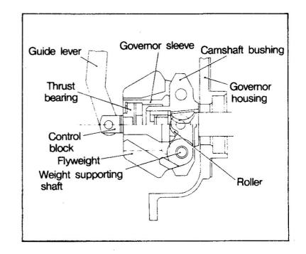
The control block, mounted to the guide lever hung on the supporting lever shaft of the governor cover, prevents rotation.
