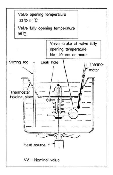
NOTE: The two thermostats in normal control trucks differ in valve opening temperature.
