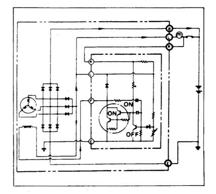
When the voltage generated by the alternator increases, the Zener diode "Dz" conducts, base current of the transistor "Tr<sub>1</sub>" flows and causes "Tr<sub>1</sub>" to be ON.
