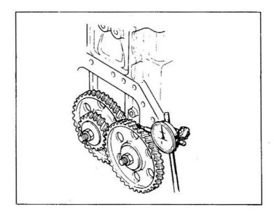
(4) Measure the idler gear and camshaft gear end plays with a thickness gauge and dial indicator. If the readings are over the repair limit, replace the thrust plate.
