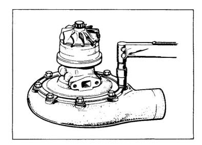
(12) Install the turbine housing 1 by tightening the bolts to the specified torque.
