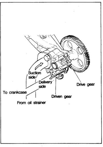
Since the oil pump is driven at speed proportional to the engine speed, the delivery pressure of the oil pump might rise excessively and overload the lubrication system during cold starting, etc. To prevent overloading the lubricating system, the oil pump has a built-in relief valve.
