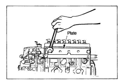
(c) Install the injection pump in special tool(Universal Vice).
