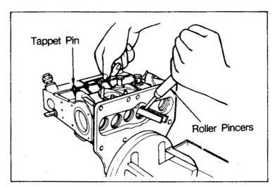
NOTE: When the camshaft is inserted, face the inscribed line on the end of the camshaft toward the timer.
