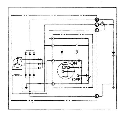
If the engine is started and the rotor excited, the stator coil generated voltage suddenly rises.
