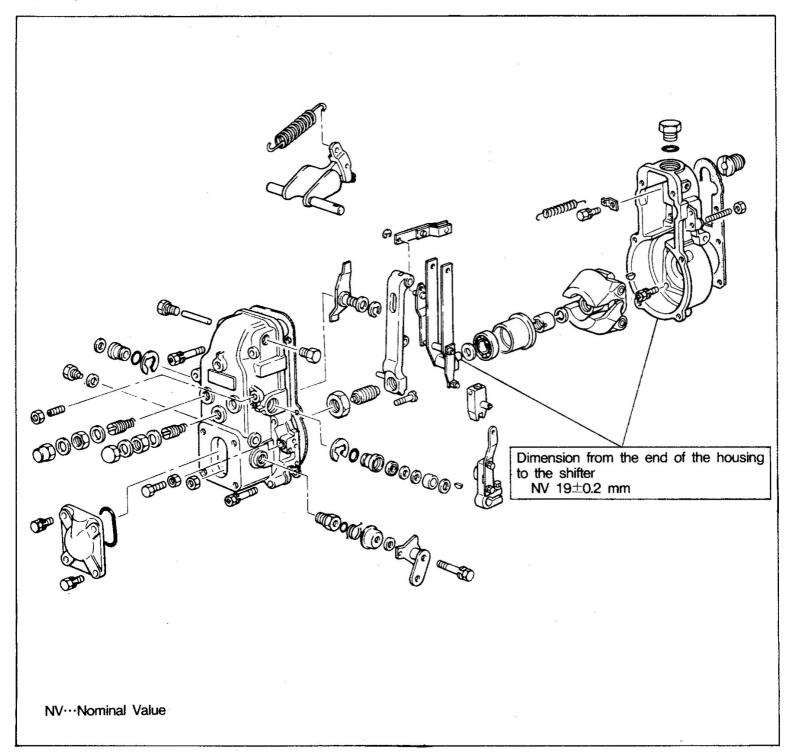
Replacement of sleeve or guide lever assembly
