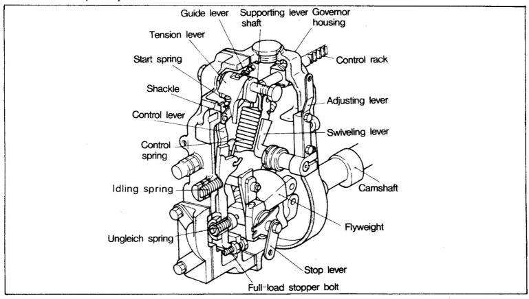
The governor, as shown, consists of flyweights mounted to the injection pump camshaft. When the flyweights turning on the flyweight supporting shaft open outward, the roller mounted to the end of flyweight arm pushes the end of the sleeve in the axial direction. The governor sleeve, being made integral with the control block through a bearing, moves only in the axial direction.
