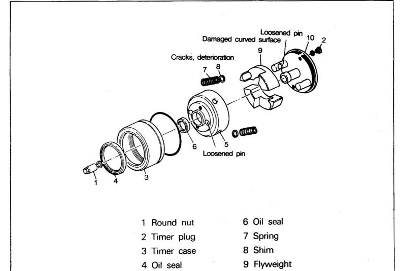
(a) Remove the coupling from the automatic timer.
