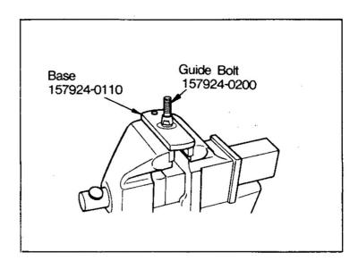
(e) Remove the timer plug 2 and place the automatic timer on special tool (Base).
