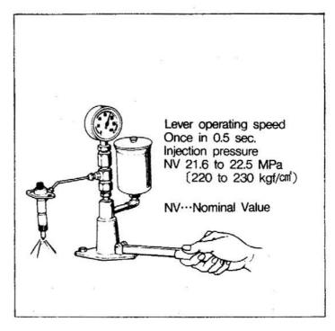
NOTE: Be sure not to touch the atomized fuel injected from the nozzle.
