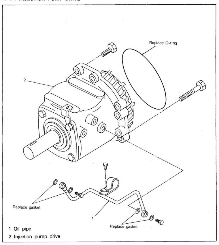
The injection pump gear mounted to the Injection pump drive must be put in correct mesh when the Injection pump drive is installed.
