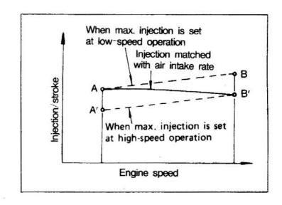
Therefore, if full load is set at point A to derive enough output at low speeds, the injection will reach B as the speed increases, and the engine will produce black smoke.
