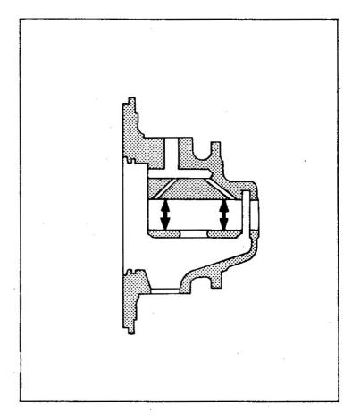
(b) Measure the shaft journal diameter. If the measured diameter is less than the service limit, replace the turbine wheel shaft.
