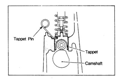
(g) Measure the end play of the camshaft with special tool(Measuring Device). If the end play is in excess of the repair limit, adjust by using shims or replace the bearing.
