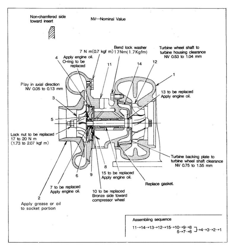
NOTE: After an overhauled turbo charger has been installed to the engine, run the engine at low idle speed for more than three minutes.
