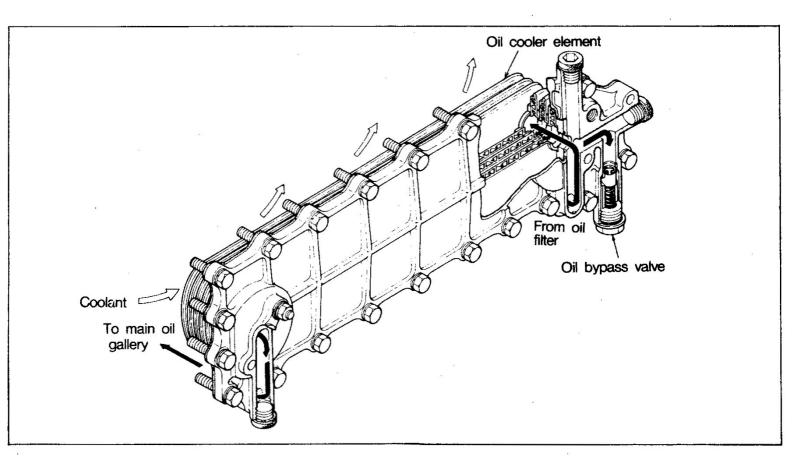
When the oil viscosity is high at low temperatures or when the element is clogged and the element has high resistance to flow, the oil bypass valve provided at the oil cooler opens so that the engine oil flows to the main gallery without passing through the oil cooler.
