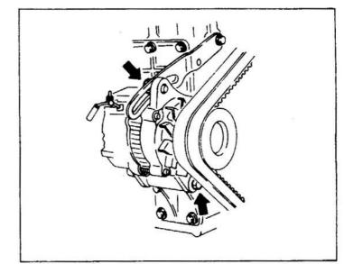
Slightly loosen the tension pulley nut and turn the adjusting bolt to adjust the belt tension.
