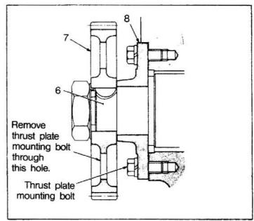
(6) Remove the lock nut and lock washer of the camshaft gear and withdraw the camshaft gear 7 with Gear Puller(special tool).
