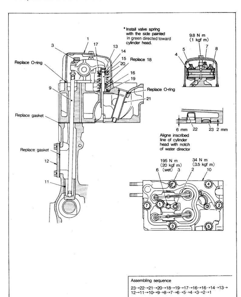
Install the sealing cap 23 and water director 22 in the cylinder head.
