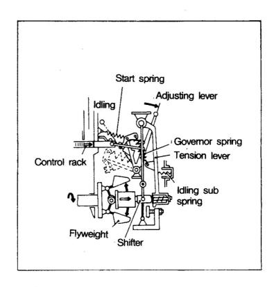
When the speed falls, the centrifugl force decreases, the flyweights move inward, and the idling sub spring pushes the tension lever to the left and moves the control rack in the direction that fuel is increased.
