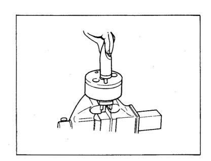
(j) After the automatic timer has been installed on the camshaft, fit special tool (Special Spanner) into the coupling mounting hole. While holding it to prevent turning, tighten the round nut 1 to the specified torque.
