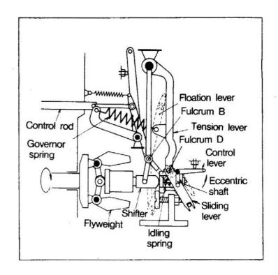
As the engine speed increases, the centrifugal force of the flyweight will increase, and the flyweight will push the shifter. In the normal speed range, however, the shifter will have only a thrust enough for compressing the idling spring and will not be able to push the tension lever out by overcoming the tension of the governor spring.
