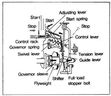
At the same time, the control block and governor sleeve push the flyweight roller to the left.
