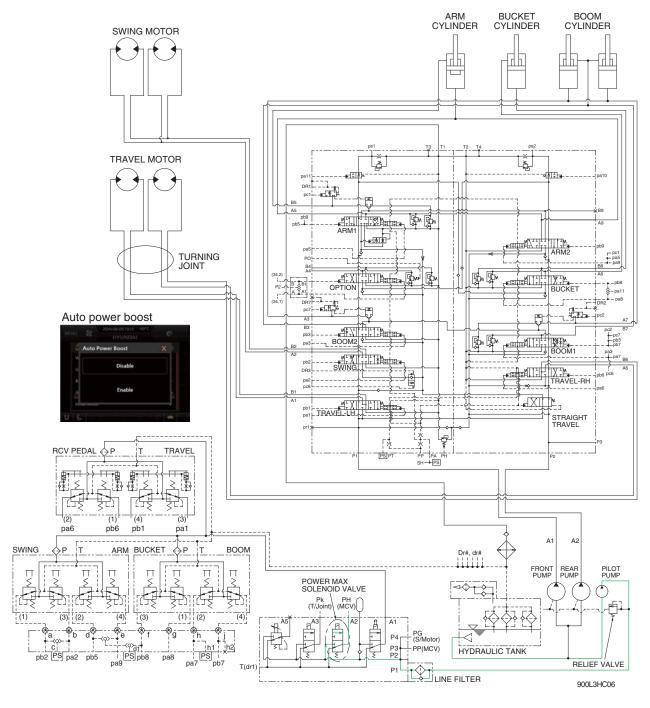
When the power max switch on the left control lever is pushed ON, the power max solenoid valve is actuated, the discharged oil from the pilot pump flow into PH port of the main relief valve of main control valve; Then the setting pressure of the main control valve is raises from 330 kgf/cm² (4690 psi) to 360 kgf/cm² (5120 psi) for increasing the digging power. And even when press continuously, it is canceled after 8 seconds.
