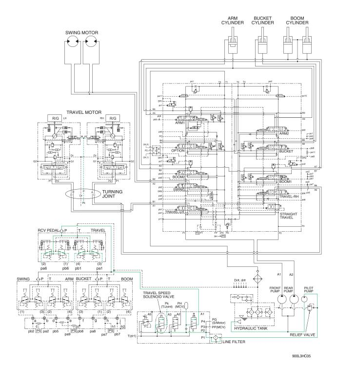
When the travel speed switch is pushed, the travel speed solenoid valve is actuated and the discharged oil from the pilot pump flows to the **Pi** port of pilot valve in the travel motors.
