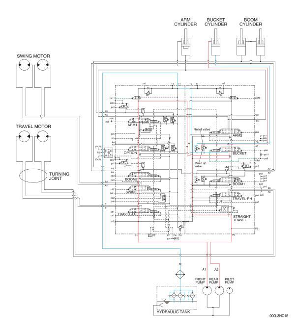
When the RH control lever is pushed right, the bucket spool in the main control valve is moved to the roll out position by the pilot oil pressure from the remote control valve.
