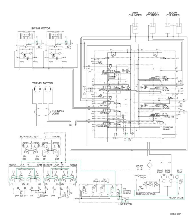
When one of the RCV lever (except travel lever) is tilted, the pilot oil flows into SH port through main control valve.
