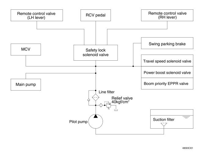
The pilot circuit consists of suction circuit, delivery circuit and return circuit.
