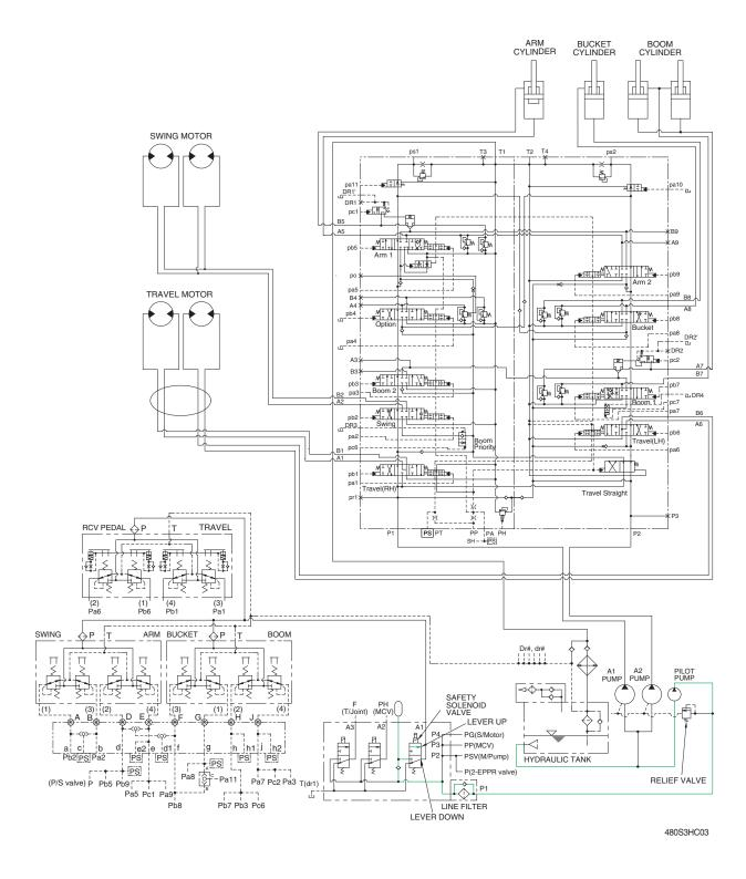
When the lever of the safety solenoid valve is moved downward, oil flows into the remote control valve through solenoid valve and line filter.
