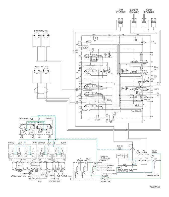
The pilot pump receive oil from the hydraulic tank. The discharged oil from the pilot pump flows to the safety solenoid valve through the line filter. The oil is filtered by the line filter. The pilot relief valve is provided in the pilot pump for limiting the pilot circuit pressure.
