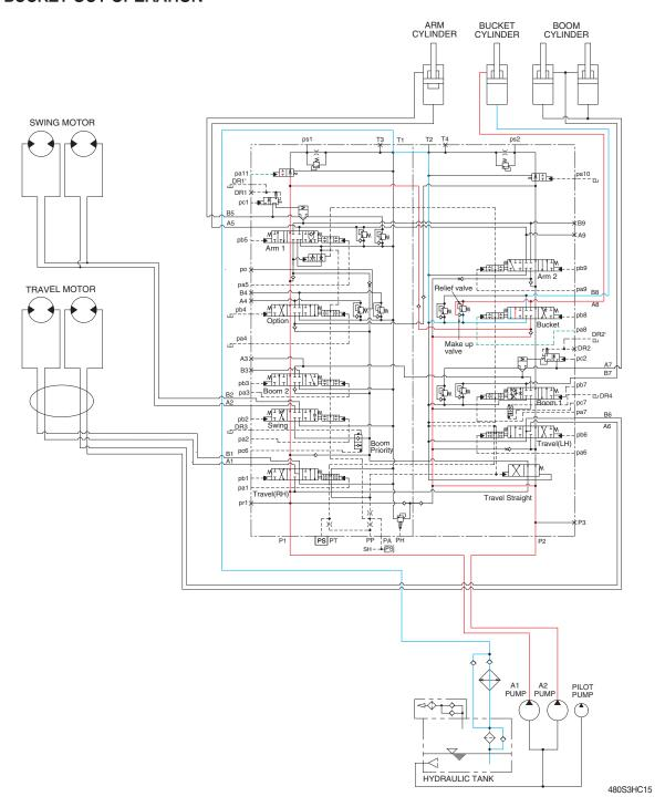
When the RH control lever is pushed right, the bucket spool in the main control valve is moved to the roll out position by the pilot oil pressure from the remote control valve.
