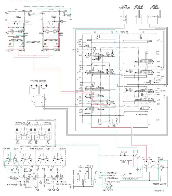
When the LH control lever is pushed left or right, the swing spool in the main control valve is moved to the left or right swing position by the pilot oil pressure from the remote control valve.
