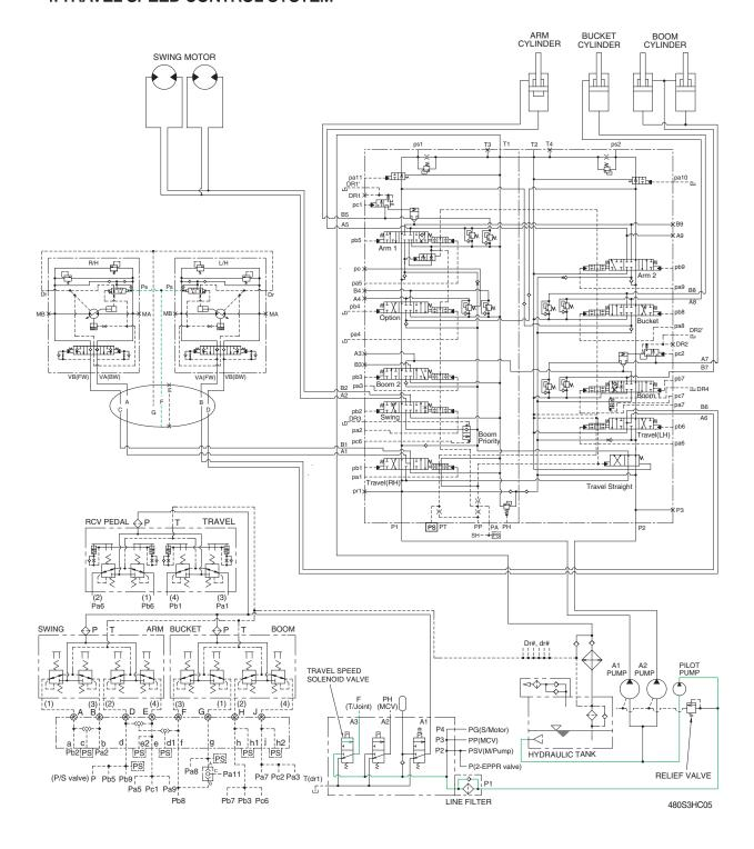
When the travel speed solenoid valve was placed in the Hi position, the pressure oil from pilot pump through line filter flows to port **Ps** of travel speed change over valve, and the control piston is pushed up, thus minimizing the displacement.
