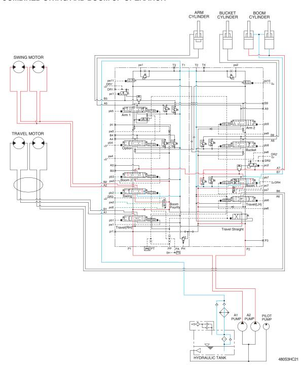
When the swing and boom up functions are operated, simultaneously the swing spool and boom spools in the main control valve are moved to the functional position by the pilot oil pressure from the remote control valve.
