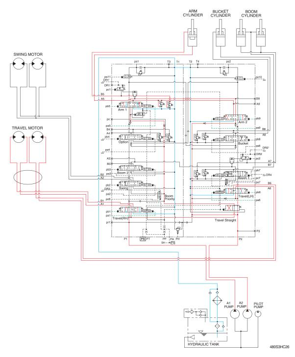
When the arm and travel functions are operated, simultaneously the arm spools and travel spools in the main control valve are moved to the functional position by the pilot oil pressure from the remote control valve and the straight travel spool is pushed to the right by the oil pressure from pilot pump.
