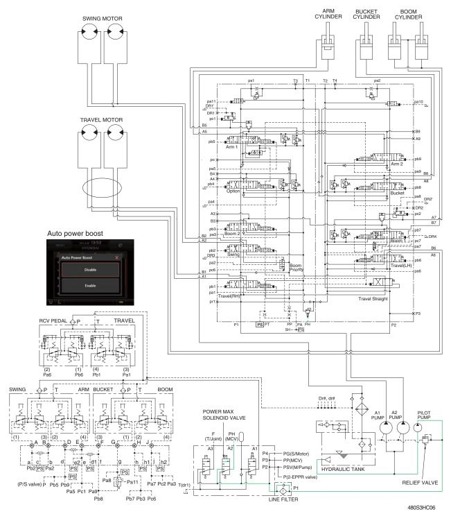
When the power max switch on the left control lever is pushed ON, the power max solenoid valve is actuated, the discharged oil from the pilot pump into PH port of the main relief valve of main control valve; Then the setting pressure of the main control valve is raises from 330 kgf/cm² to 360 kgf/cm² for increasing the digging power. And even when press continuously, it is canceled after 8 seconds.
