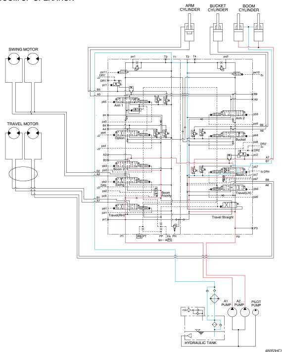
When the RH control lever is pulled back, the boom spools in the main control valve are moved to the up position by the pilot oil pressure from the remote control valve.
