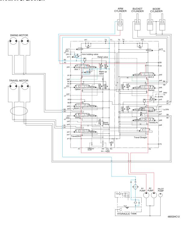
When the LH control lever is pulled back, the arm spools in the main control valve are moved the to roll in position by the pilot oil pressure from the remote control valve.
