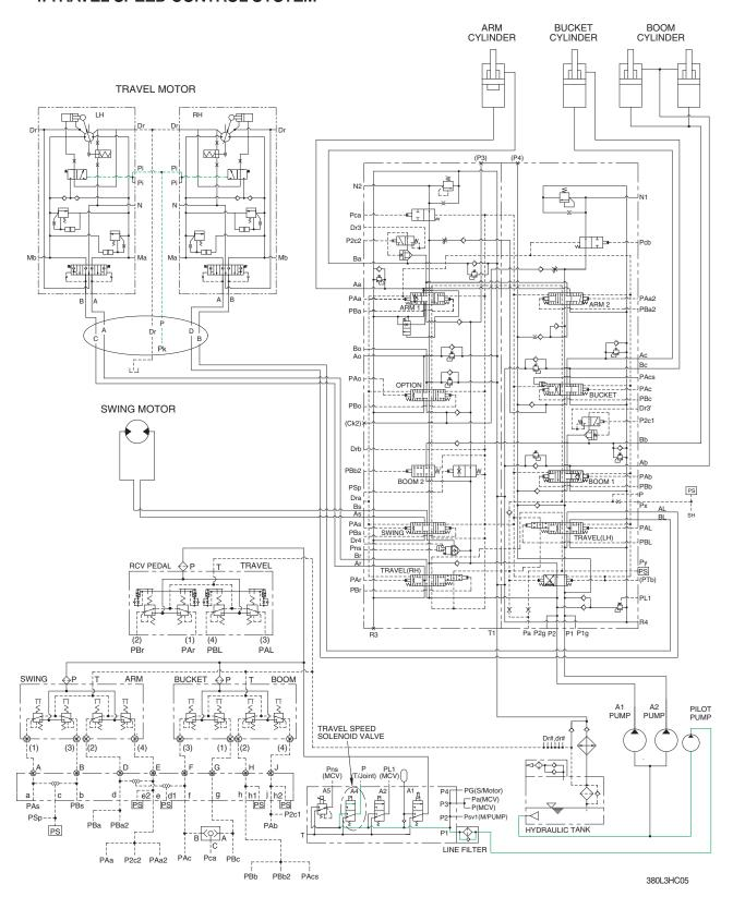
When the travel speed solenoid valve was placed in the Hi position, the pressure oil from pilot pump through line filter flows to port **Pi** of travel speed change over valve, and the control piston is pushed left (LH) and right (RH), thus minimizing the displacement.
