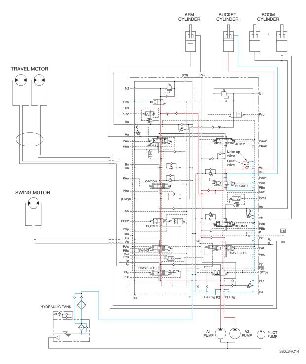
When the RH control lever is pulled left, the bucket spool in the main control valve is moved to the roll in position by the pilot oil pressure from the remote control valve.
