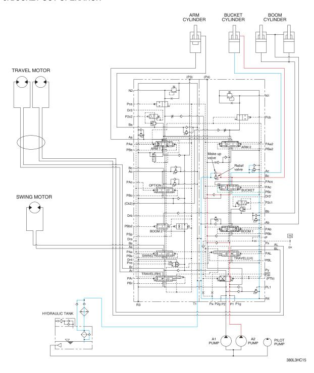
When the RH control lever is pushed right, the bucket spool in the main control valve is moved to the roll out position by the pilot oil pressure from the remote control valve.
