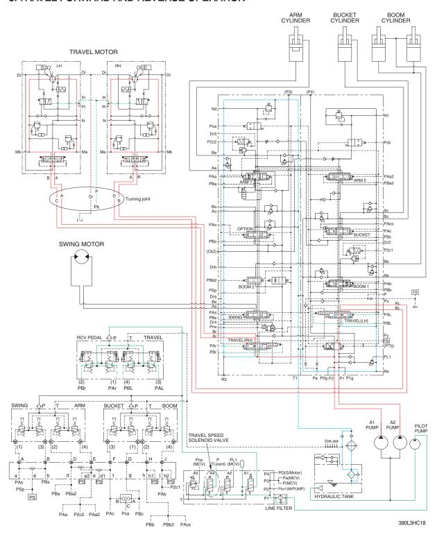
When the travel levers are pushed forward or reverse position, the travel spools in the main control valve are moved to the forward or reverse travel position by the pilot oil pressure from the remote control valve.
