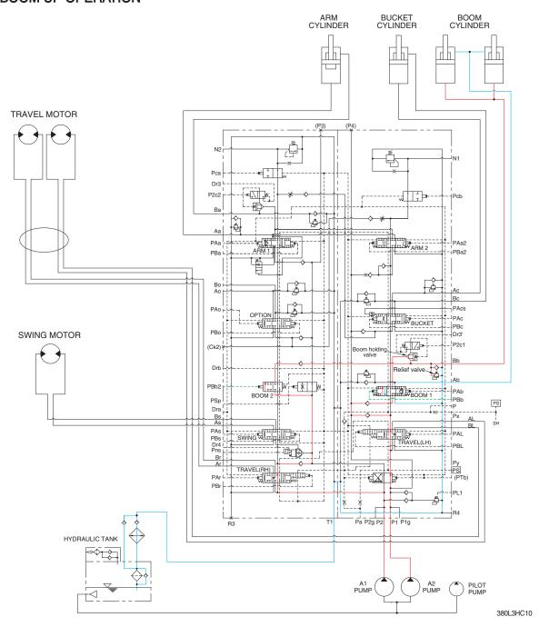
When the RH control lever is pulled back, the boom spools in the main control valve are moved to the up position by the pilot oil pressure from the remote control valve.
