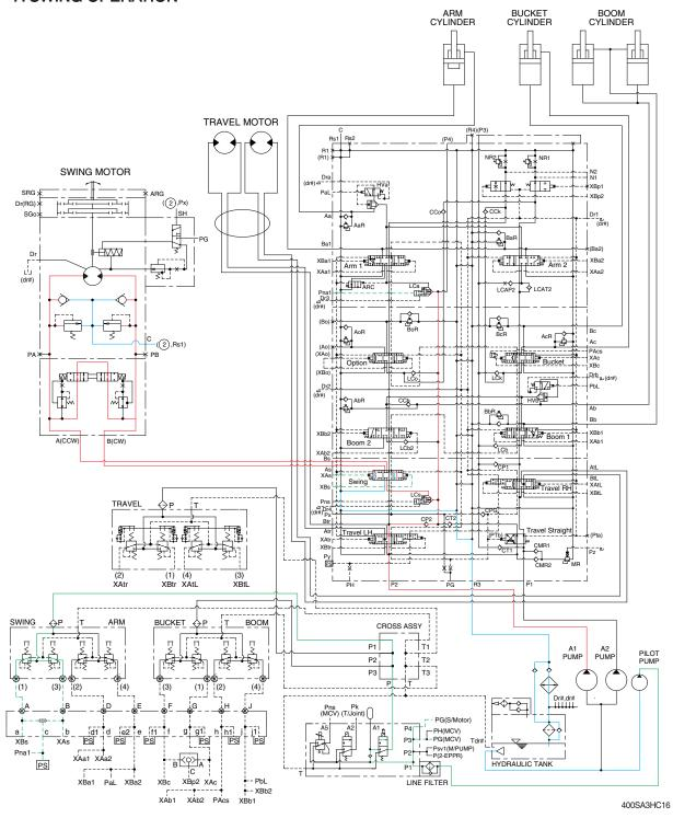
When the LH control lever is pushed left or right, the swing spool in the main control valve is moved to the left or right swing position by the pilot oil pressure (XAs, XBs) from the remote control valve.
