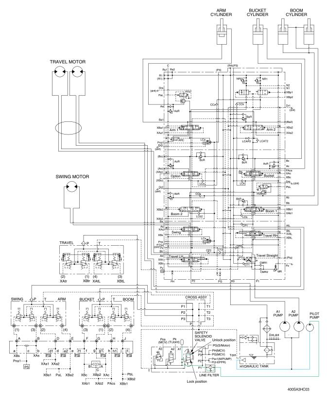
When the knob of the safety solenoid valve is turned to the unlock position, oil flows into the remote control valve through line filter, safety solenoid valve and cross assy.
