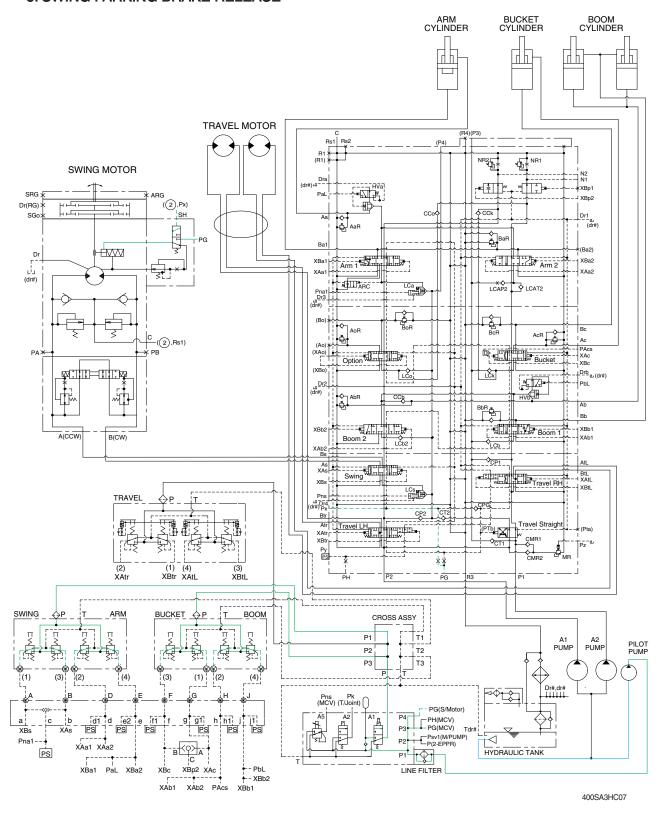
When one of the RCV lever (except travel lever) is tilted, the pilot oil flows into SH port through main control valve (Px).
