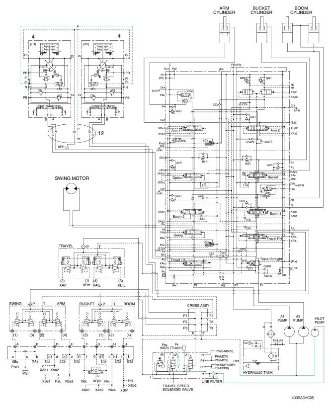
When the travel speed solenoid valve was placed in the Hi position, the pressure oil from pilot pump through line filter flows to port **Pi** of travel speed change over valve, and the control piston is pushed left (RH) and right (LH), thus minimizing the displacement.
