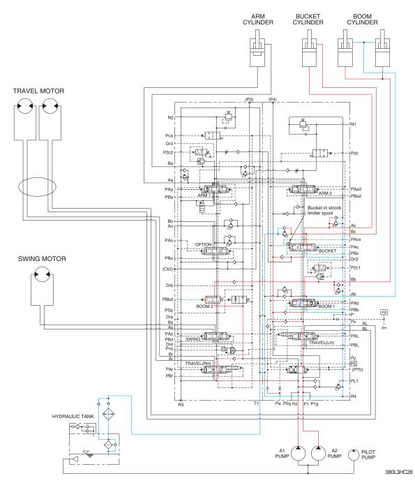
When the boom up and bucket functions are operated simultaneously, each spool in the main control valve is moved to the functional position by the pilot oil pressure from the remote control valve. The oil from the A1 pump flows into the boom cylinders through the boom 2 spool in the left control valve. The oil from the A2 pump flows into the boom cylinders and bucket cylinder through the boom 1 spool, bucket spool and the parallel and confluence oil passage in the right control valve.
