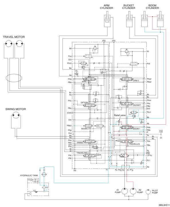
When the RH control lever is pushed forward, the boom 1 spool in the main control valve is moved to the down position by the pilot oil pressure from the remote control valve.
