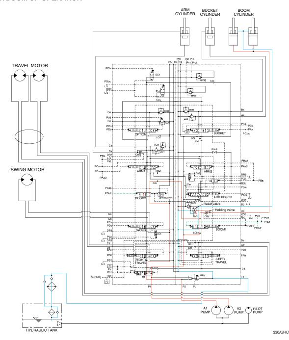
When the right control lever is pulled back, the boom spools in the main control valve are moved to the up position by the pilot oil pressure (PBb1, PDb2) from the remote control valve.
