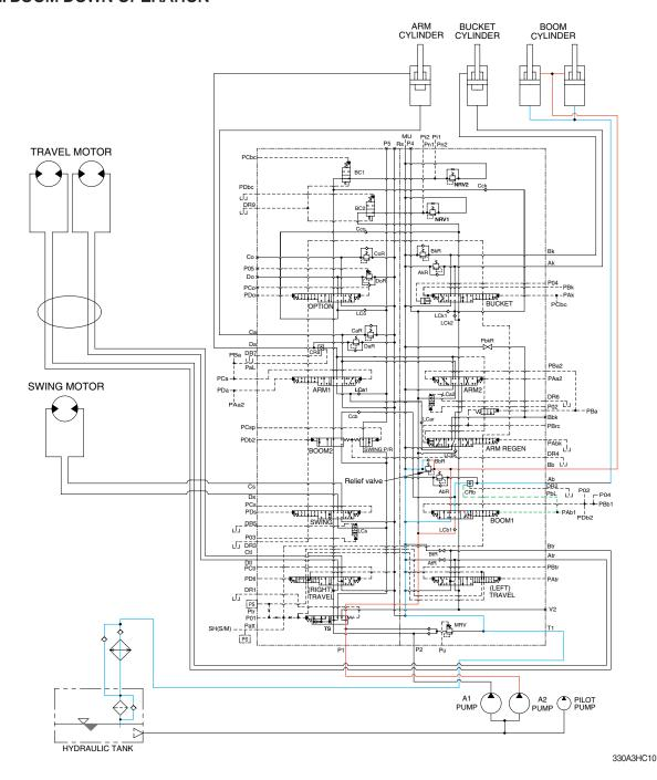
When the right control lever is pushed forward, the boom 1 spool in the main control valve is moved to the down position by the pilot oil pressure (PAb1) from the remote control valve.
