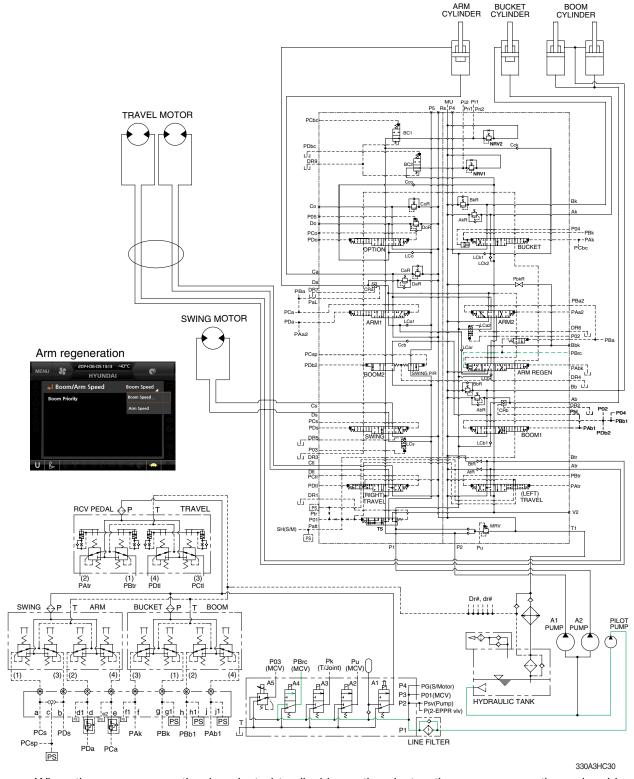
When the arm regeneration is selected to disable on the cluster, the arm regeneration solenoid valve is activated. The pilot oil from pilot pump flow into **PBrc** port in main control valve through solenoid valve and the arm regeneration spool is shifted to right.
