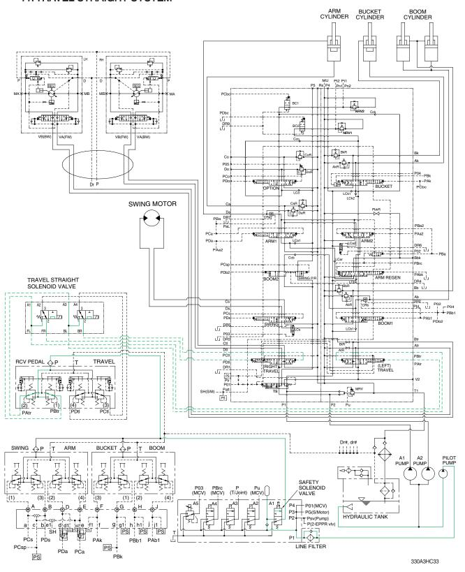
When the travel straight switch on the switch panel is pressed ON position, the travel straight solenoid valves are activated. The pilot oil from the left travel control valve flow into the left travel spool and right travel spool by the internal connection of the travel straight solenoid valve. Then the travel straight operation is available by the left travel pedal.
