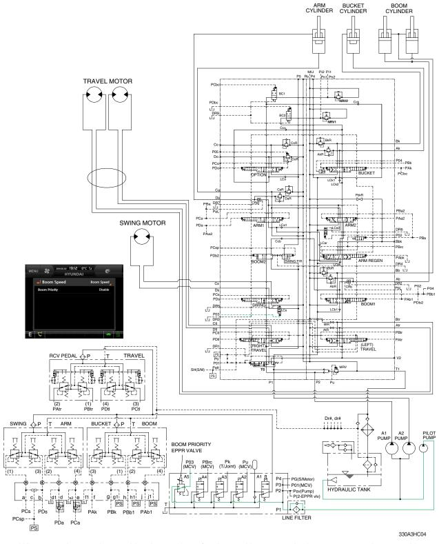
When carrying out the combined operation of swing and boom up, the boom up operating speed is lowered then normal operation.
