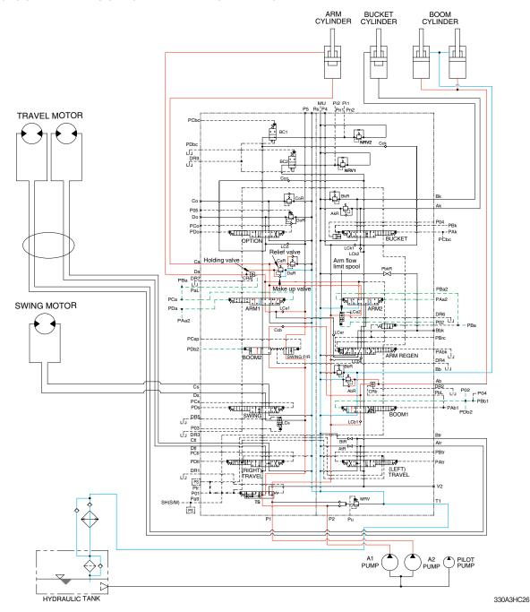
When the boom up and arm functions are operated, simultaneously each spool in the main control valve is moved to the functional position by the pilot oil pressure (PBb1, PDb1, PCa, PDa, PAa2, PBa2) from the remote control valve.
