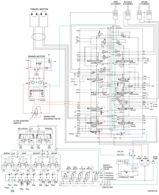
When the free/fine swing switch on the switch panel is pressed ON position, the swing fine solenoid valve is activated . The main pump side passage of the swing motor is connected to the return passage and some oil of the pump passage flows to the return passage through the swing fine solenoid and the flow oil quantity controlled by orifice.
