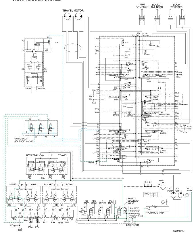
When the swing lock switch on the switch panel is pressed ON position, the swing lock solenoid valves are activated. The pilot oil from swing remote control valve to the swing spool and swing brake release shut off and the swing spool and swing brake release pilot LOCK port connect to the hydraulic tank.
