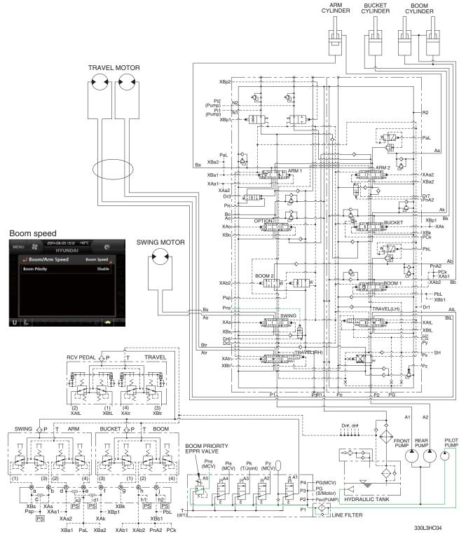
When carrying out the combined operation of swing and boom up, the boom up operating speed is lowered then normal operation.
