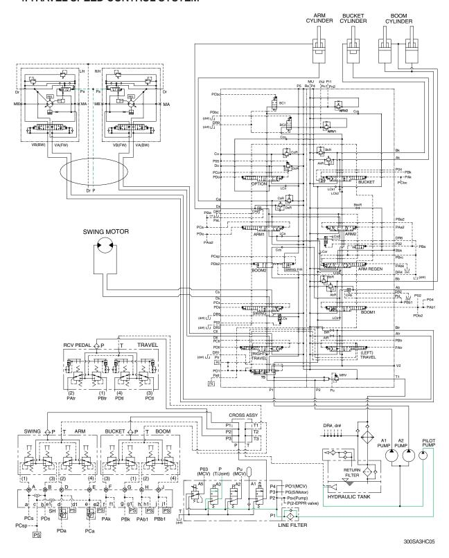
When the travel speed solenoid valve was placed in the Hi position, the pressure oil from pilot pump through line filter flows to port **Ps** of travel speed change over valve, and the control piston is pushed, thus minimizing the displacement.
