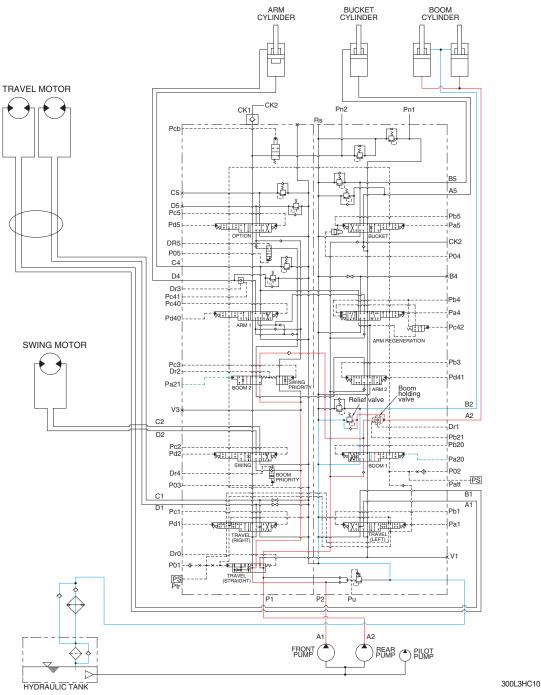
When the RH control lever is pulled back, the boom spools in the main control valve are moved to the up position by the pilot oil pressure from the remote control valve.
