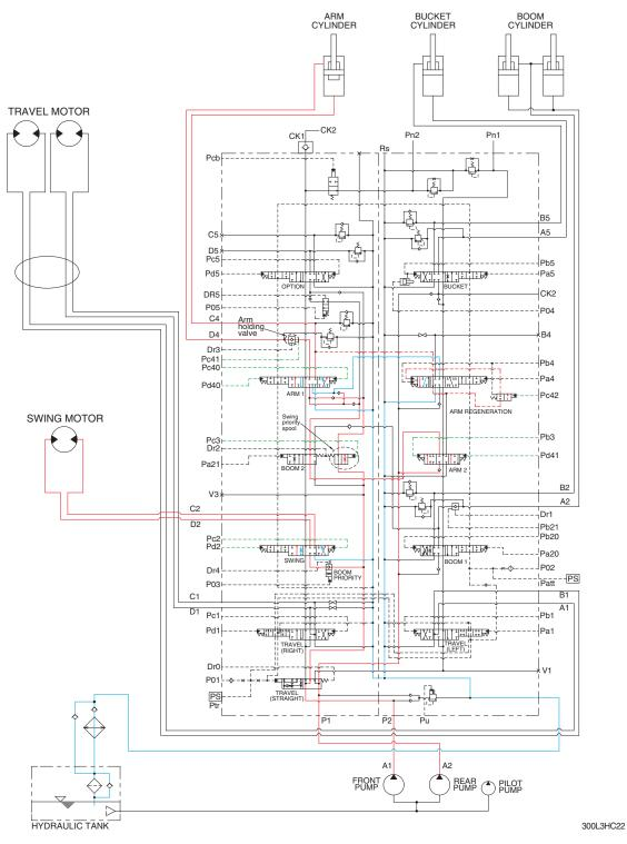
When the swing and arm functions are operated, simultaneously the swing spool and arm spools in the main control valve are moved to the functional position by the pilot oil pressure from the remote control valve.
