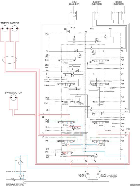
When the swing and travel functions are operated, simultaneously the swing spool and travel spools in the main control valve are moved to the functional position by the pilot oil pressure from the remote control valve. At the same time, the straight travel spool is pushed to the right by the pilot oil pressure from the pilot pump.
