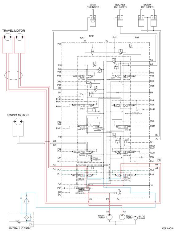
When the right and left travel levers are manually placed to the forward or reverse position, the oil flows from pilot pump through the pilot valve to travel sections of the main control valve.
