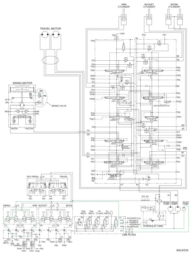
When the RCV lever (swing or arm in) is tilted, the pilot oil flows into SH port through shuttle valve. This pressure moves spool of the swing brake valve so, discharged oil from pilot valve flows to swing motor PG port.
