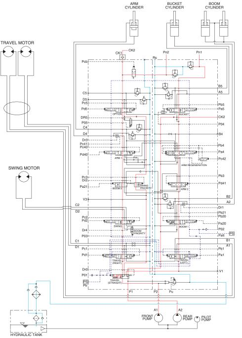
The oil from the A1 and A2 pump flows through the neutral oil passage, bypass oil passage and confluence oil passage in the main control valve. Then the oil goes to each actuator and operates them. Check valves and orifices are located on these oil passage in the main control valve. These control the oil from the main pumps so as to correspond to the operation of each actuator and smooth the combined operation.
