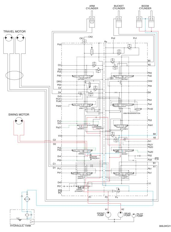
When the swing and boom up functions are operated, simultaneously the swing spool and boom spools changed. The oil flows from the A2 pump through boom 1 section of the main control valve to boom cylinders and the boom functions.
