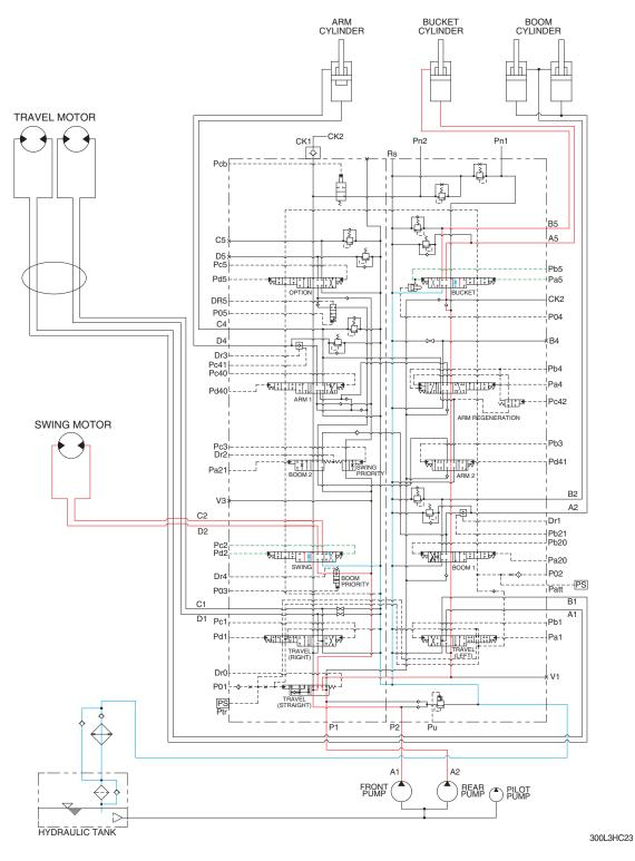
When the swing and bucket functions are operated, the swing and bucket spools changed. The oil flows from the A2 pump through the bucket section of the main control valve to the bucket cylinder and the bucket functions. The oil flows from A1 pump through swing section of the main control valve to the swing motor and swing the superstructure.
