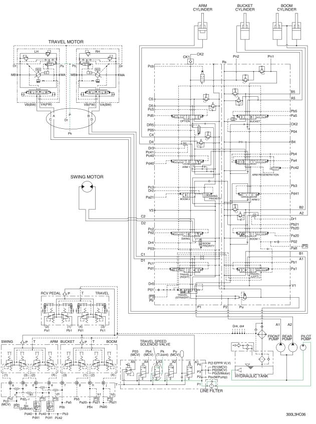
When the travel speed solenoid valve was placed in the Hi position, the pressure oil from pilot pump through line filter flows to port **Ps** of travel speed change over valve, and the control piston is pushed up, thus minimizing the displacement.
