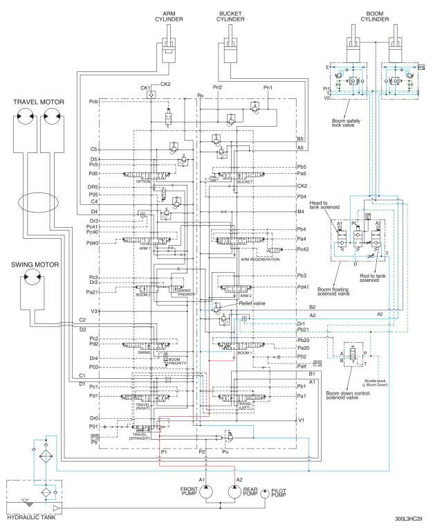
Smooth and convenient boom movement is accomplished by only arm control lever operation.
