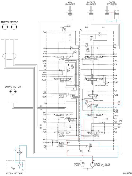
When the RH control lever is pushed forward, the boom spools in the main control valve are moved to the down position by the pilot oil pressure from the remote control valve.
