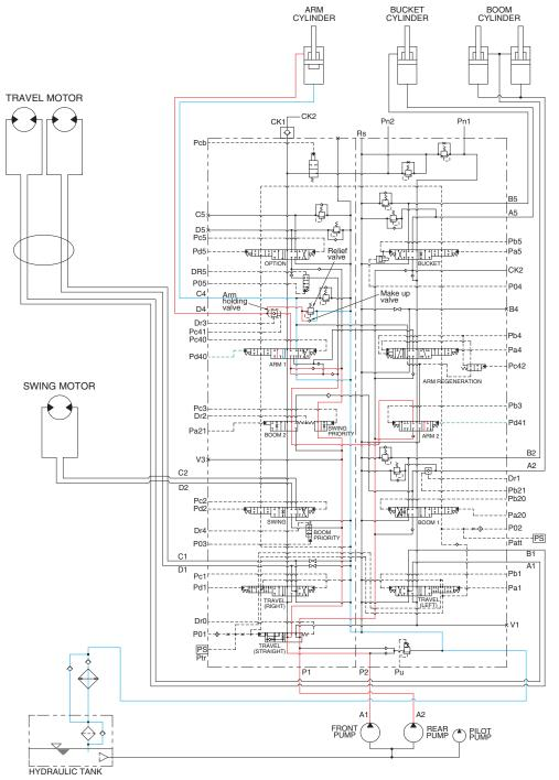
When the LH control lever is pushed forward, the arm spools in the main control valve are moved to the roll out position by the pilot oil pressure from the remote control valve.
