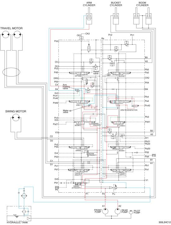
When the LH control lever is pulled back, the arm spools in the main control valve are moved to the roll in position by the pilot oil pressure from the remote control valve.
