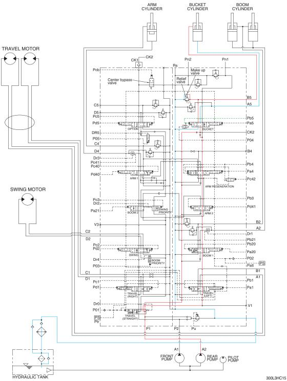
When the RH control lever is manually placed in the bucket roll out position. Then the oil flows from pilot pump through the pilot valve to bucket section of the main control valve. Here the spool position is moved to bucket roll out position.
