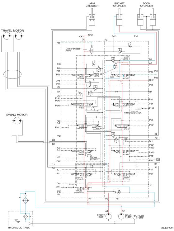
When the RH control lever is manually placed in the bucket roll in position. Then the oil flows from pilot pump through the pilot valve to bucket section of the main control valve. Here the spool position is moved to bucket roll in position.
