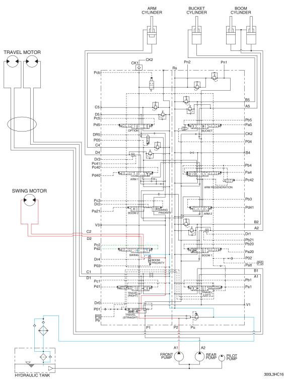
When the LH control lever is manually placed in the left (right) swing position. Then the oil flows from A1 pump through the swing section of the main control valve to swing motor to left (right) swing the superstructure. The return oil flows from swing motor through the swing section of the main control valve returned to the tank.
