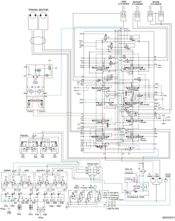
When the left control lever is pushed left or right, the swing spool in the main control valve is moved to the left or right swing position by the pilot oil pressure (PCs, PDs) from the remote control valve. Also the swing operation preference function is operated by the pilot pressure PCsp (refer to page 2-51).
