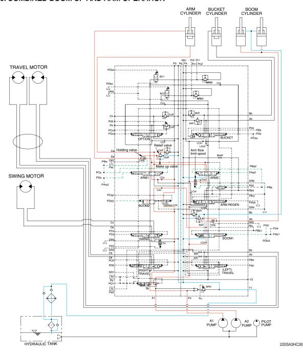
When the boom up and arm functions are operated, simultaneously each spool in the main control valve is moved to the functional position by the pilot oil pressure (PAb1, PDb2, PCa, PDa, PAa2, PBa2) from the remote control valve.
