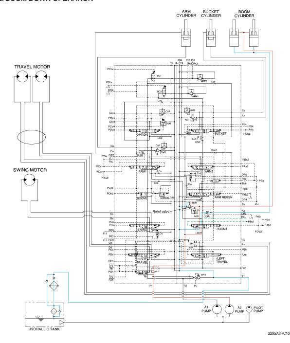
When the right control lever is pushed forward, the boom 1 spool in the main control valve is moved to the down position by the pilot oil pressure (PBb1) from the remote control valve.
