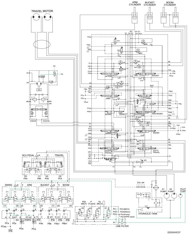
When the RCV lever (swing or arm in) is tilted, the pilot oil flows into SH port through shuttle valve. This pressure moves spool of the swing brake valve so, discharged oil from pilot valve flows to swing motor PG port. This pressure is applied to swing motor disc, thus the brake is released. When the RCV lever (swing or arm in) is set in the neutral position, oil in the swing motor disc cylinder is drained, thus the brake is applied.
