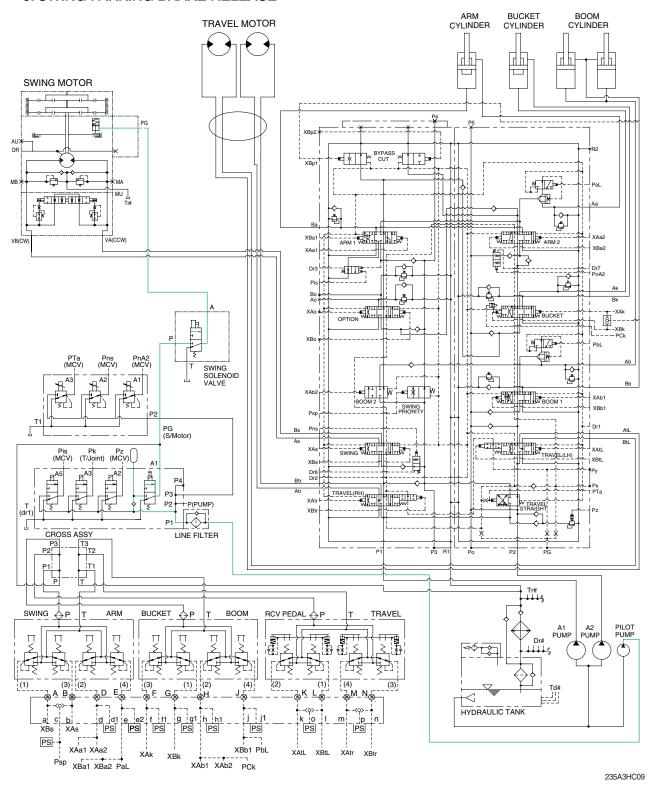
When the swing control lever is tilted, the swing solenoid valve is shifted to the down ward by the MCU that senses the pilot pressure of the swing control lever.
