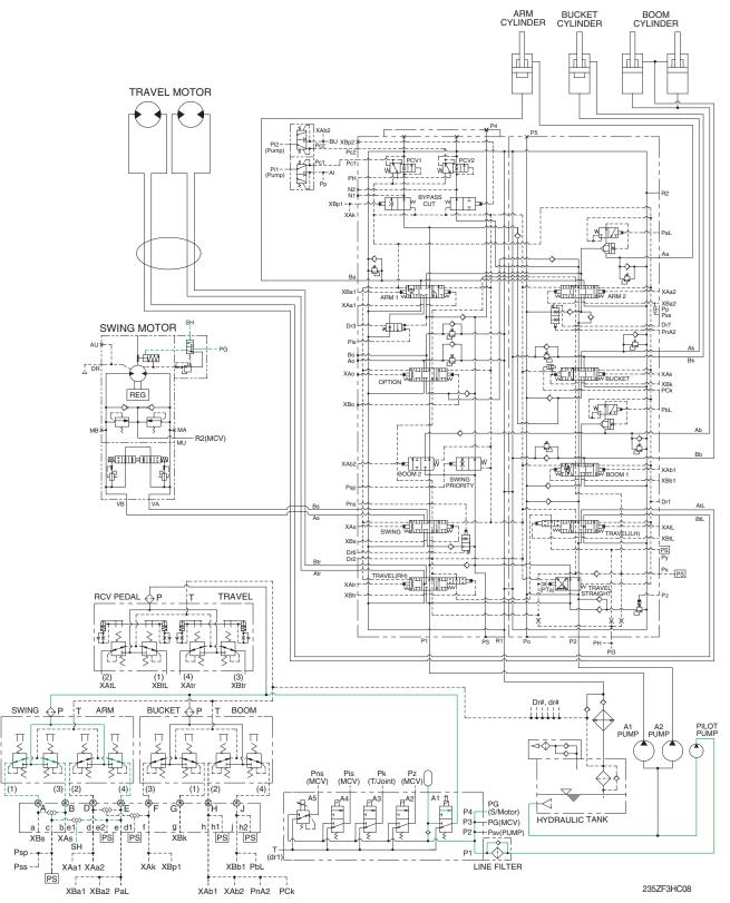
When the swing control lever or arm in control lever is tilted, the pilot oil flows into **SH** port through main control valve.
