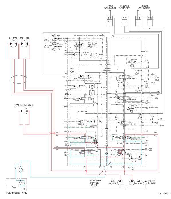
When the swing and travel functions are operated simultaneously, the swing spool and travel spools in the main control valve are moved to the functional position by the pilot oil pressure from the remote control valve and straight travel spool is pushed to the right by the pilot oil pressure from the pilot pump.
