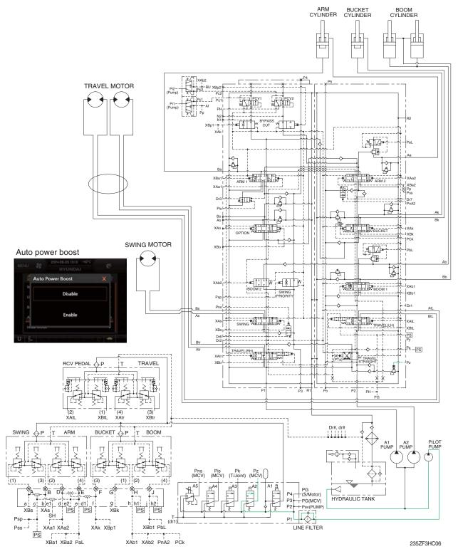
When the power boost switch on the left control lever is pushed ON, the power boost solenoid valve is actuated, the discharged oil from the pilot pump flows into **Pz** port of the main relief valve of main control valve; then the setting pressure of the main relief valve is raised from 350 kgf/cm<sup>2</sup> (4980 psi) to 380 kgf/cm<sup>2</sup> (5400 psi) for increasing the digging power.
