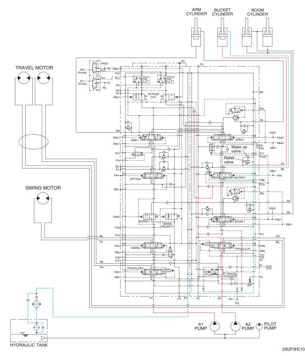
When the right control lever is pulled left, the bucket spool in the main control valve is moved to the
