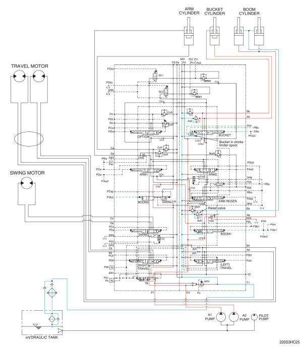
When the boom up and bucket functions are operated, simultaneously each spool in the main control valve is moved to the functional position by the pilot oil pressure from the remote control valve.
