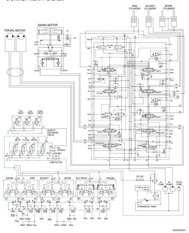
When carrying out the combined operation of swing and arm of the left control valve, the swing speed can be lowered than operating speed of arm.
