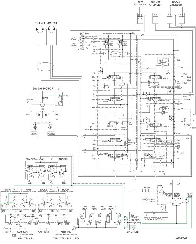
When one of the RCV lever (except travel lever) is tilted, the pilot oil flows into SH port through shuttle valve.
